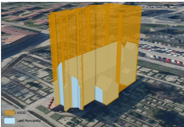
Figure 4.6: Building 6 of the VGI3D (orange) and Lund municipality (blue) models. These two buildings have the second-largest difference in volume and envelope area of any building. The substantial size difference is likely because the building has unusual shapes and window geometry.
