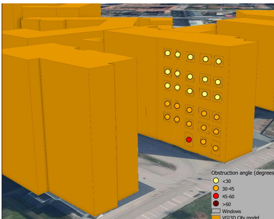
Figure 3.9: Visualization of the obstruction angle tools output on the VGI3D city model.
