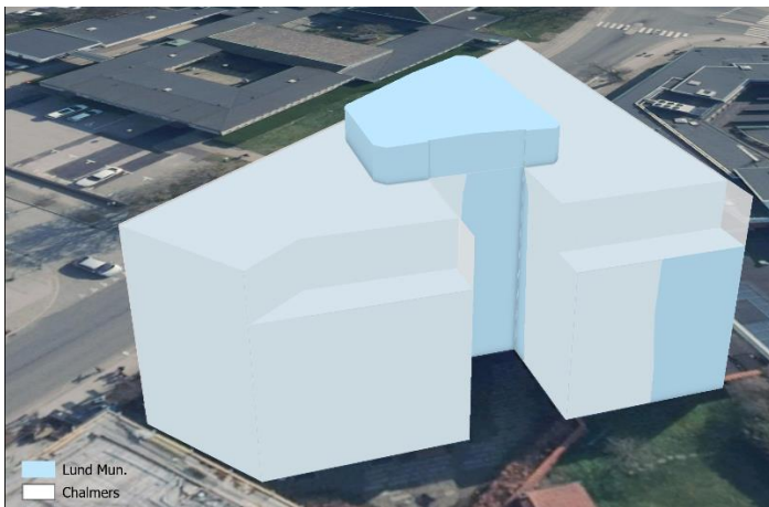
Figure 4.5: Building 5 of the Lund municipality (blue) and Chalmers (white) models. These are the buildings with the smallest difference in volume.
