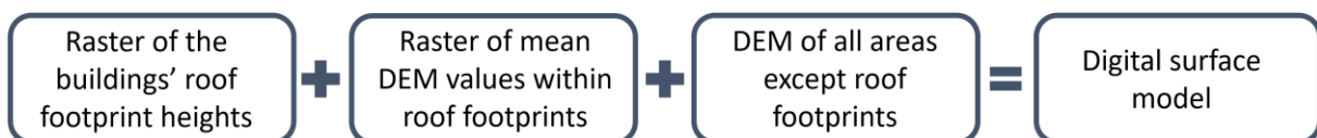
Figure 3.3: An illustration of how the DSMs for each 3D city model were created.
