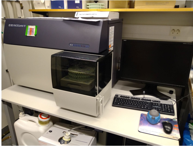
Figure 2.2: Fluorescence Activated Cell Sorting used to analyse the stained tumor samples.
