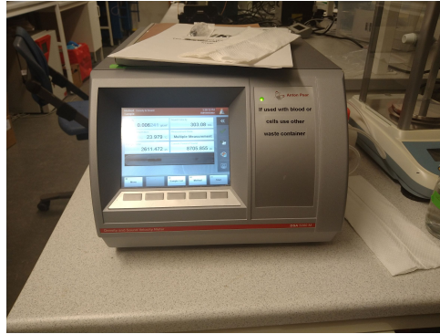
Figure 2.8: The Density and sound velocity meter DSA 5000 M from Anton Paar used to measure the densities of the mediums used in the experiments.
