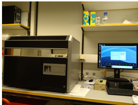
Figure 2.9: The Amnis ImagestreamX-MKII which was used to measure the size of the tumor cells
