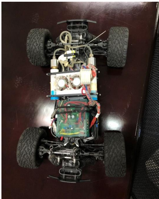
Images 1 and 2: Hydrogen fuel-cell car prototype; and miniature hydrogen fuel cell charger. Both objects are teaching material used by ACH2. The researcher took photos during a field trip.
