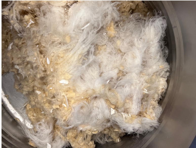
(a) 51mm bico-fibers mixed with shredded wool
