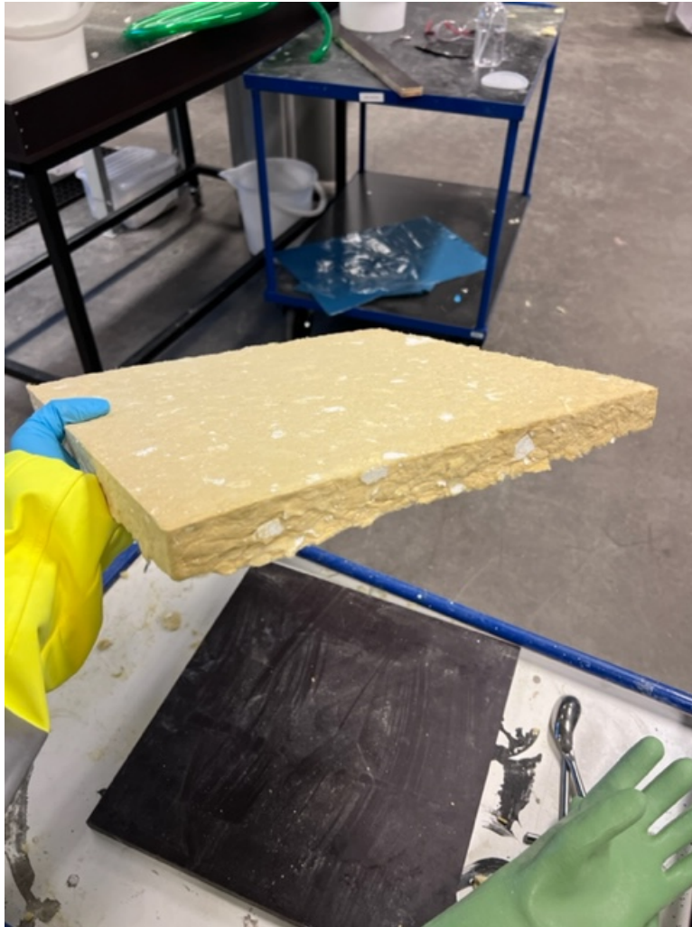
Figure 6.6: Prototype with high density made from fine shredded wool with phenolic binder
