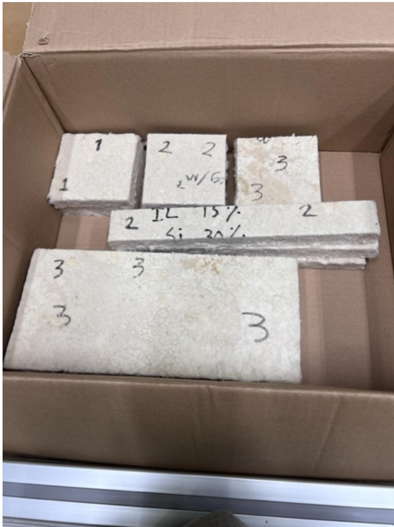
Figure 6.3: Cut samples for fire, mechanical and acoustic tests.
