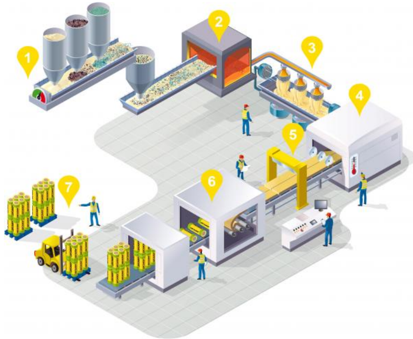
Figure 3.18: The process for glass wool manufacturing at Isover Saint-Gobain [18]
