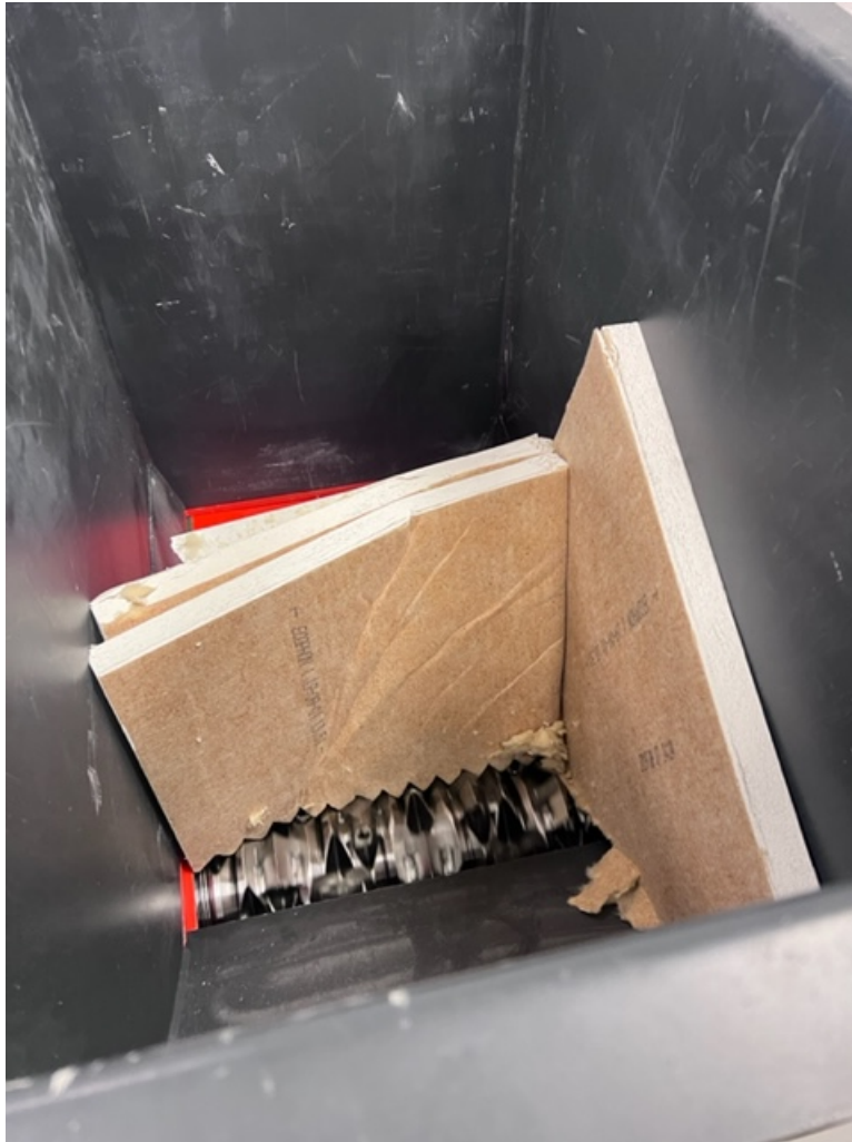
Figure 5.2: Acoustic tiles in shredder, at TLF varberg
