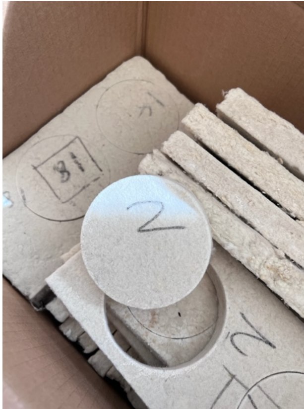
Figure 6.4: Cut samples for AFR measurements.
