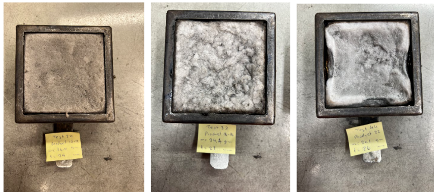
Figure 7.9: The same samples after the fire test
