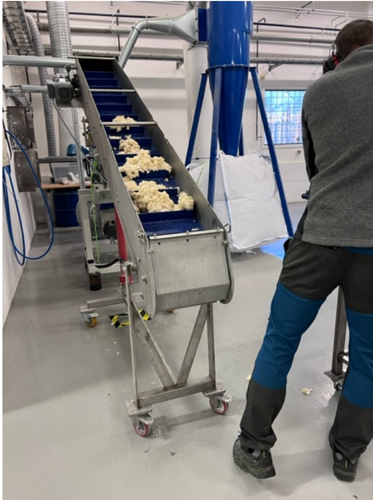
Figure 5.3: Shredded wool put on a moving band into the hammer mill.
