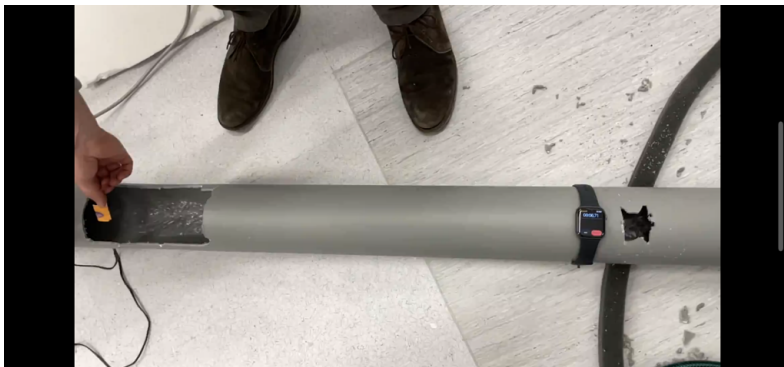
Figure B.5: The setup while measuring the surface flow velocity with slow motion camera and the Apple Watch in the Acconeer lab environment.
