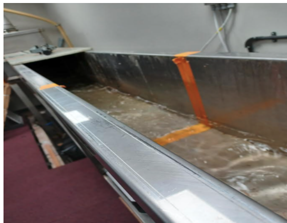
Figure 3.5: Water flow in the rectangular open channel on UK lab site.
