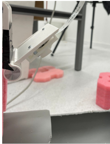
Figure 3.3: The figure shows the sensor further up above the water surface compared to the setup in figure 3.2 . An increased distance from sensor to water surface enables the use of a different profile setting.
