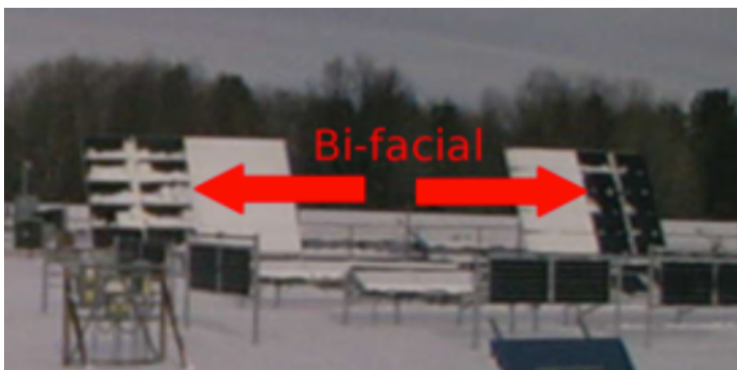
Figure 9. The bifacial modules (partly snow free) in this setup shed snow faster than the monofacial modules (snow covered). The bifacial modules on the left are framed while the bifacial modules on the right are frameless. Source: (Burnham et al., 2019b)
