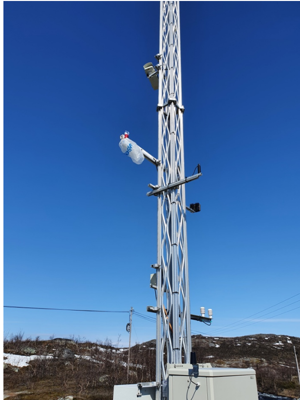
Figure 17. The pyranometer is mounted S-SE on the mast of Vegvesenet, next to Gálggojávri. The pyranometer is the black vertical cylinder on the right hand side of the mast. Source: (Boström, 2022a)
