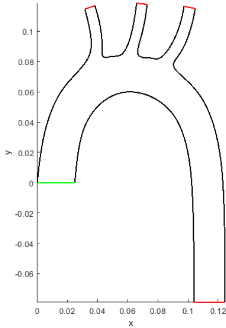
Figure 3.3: Aorta geometry. Green represents inlet, red outlets and black is the walls.
