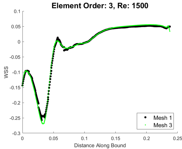
Figure 4.4: Comparison of the wall shear stress along the lower wall of the aorta mesh for the coarsest mesh (mesh 1) and the finest mesh (Mesh 3) using an element order of 3 and Reynolds number of 1500
