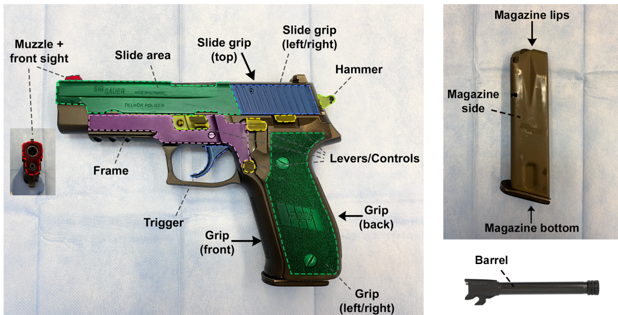
Figure 10: the different areas of the police officers' practice weapon that were swabbed. The figure shows the left side of the pistol and right side of the magazine. The barrel is found inside the pistol.
