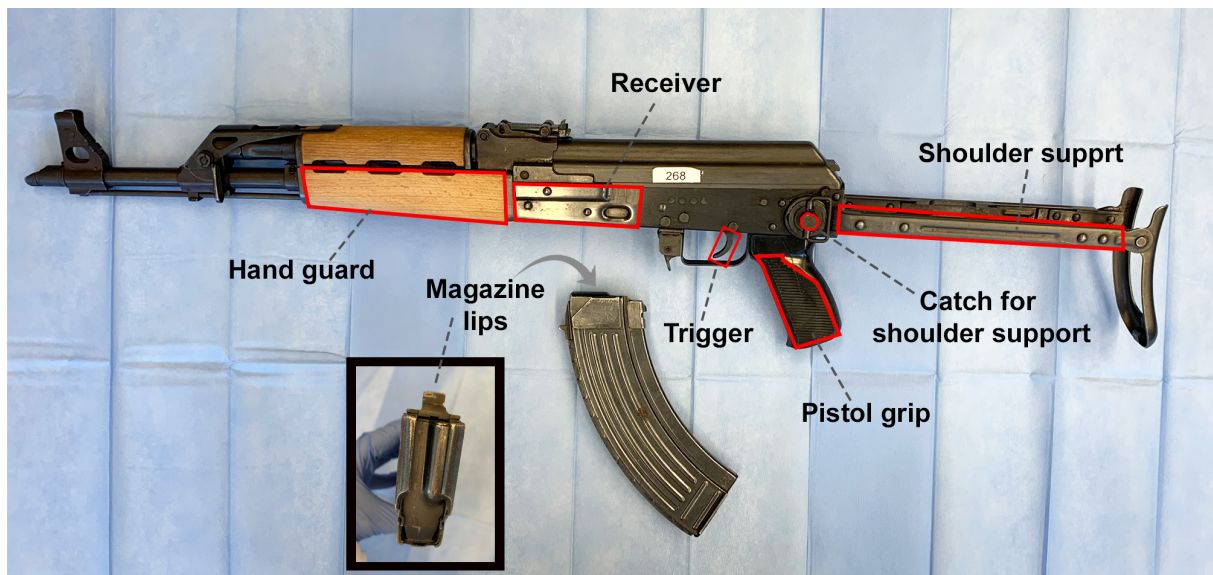
Figure 7: the different areas of the Kalashnikov that were swabbed for the swab study with saliva.
