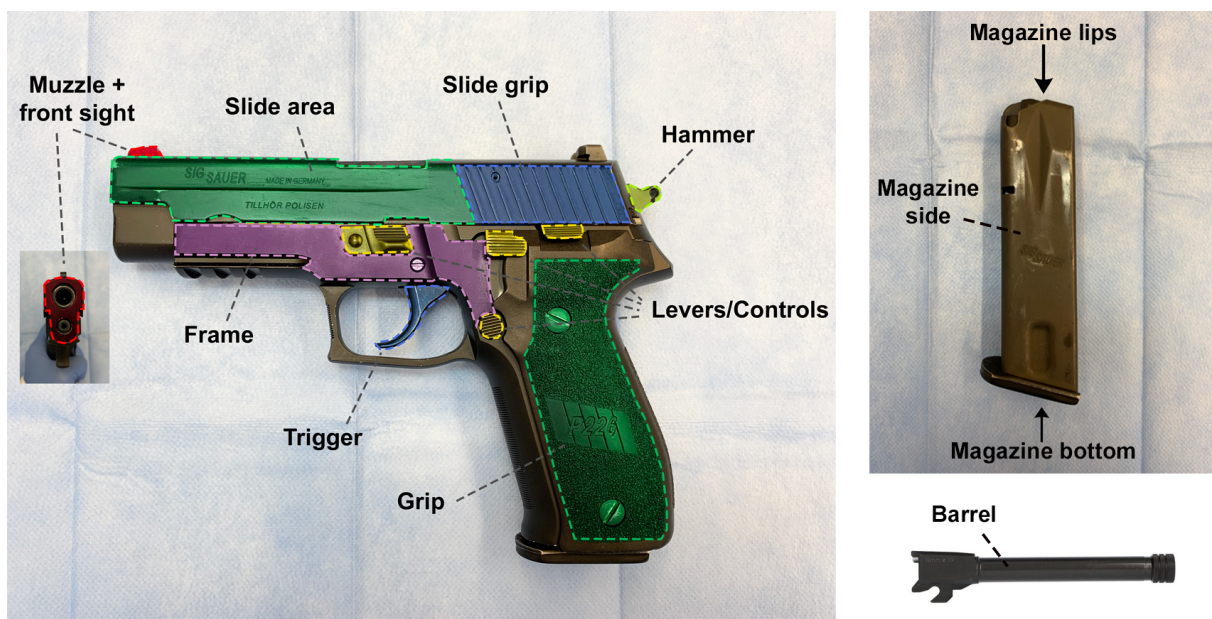
Figure 9: the different areas of the crime scene investigators’ service weapons that were swabbed. The figure shows the left side of the pistol and the right side of the magazine. The barrel is found inside the pistol.
