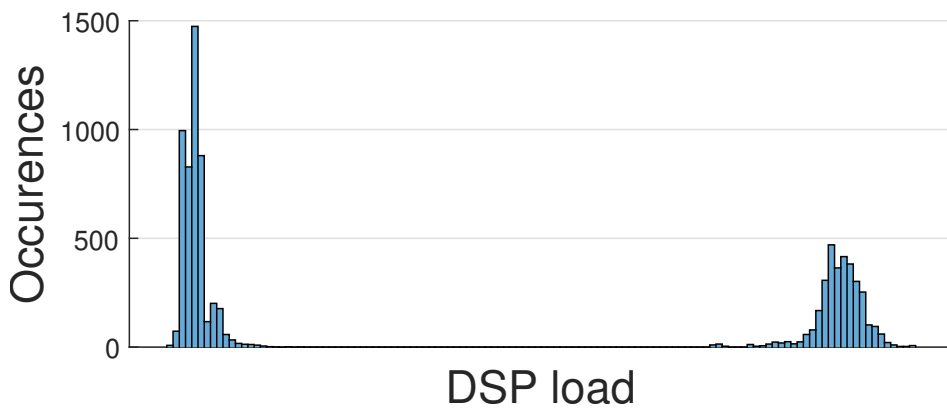
Figure A.10: Histogram for DSP load measurements. Three sectors and a 50 MHz cell.
