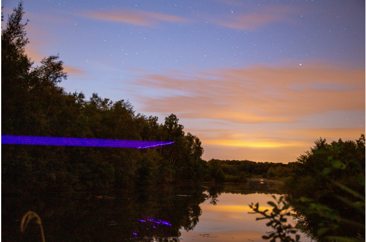
Figure 34: Inelastic hyperspectral lidar using a laser beam at 405 nm which scans a forest area and measures the induced fluorescent emission of the chlorophyll.
