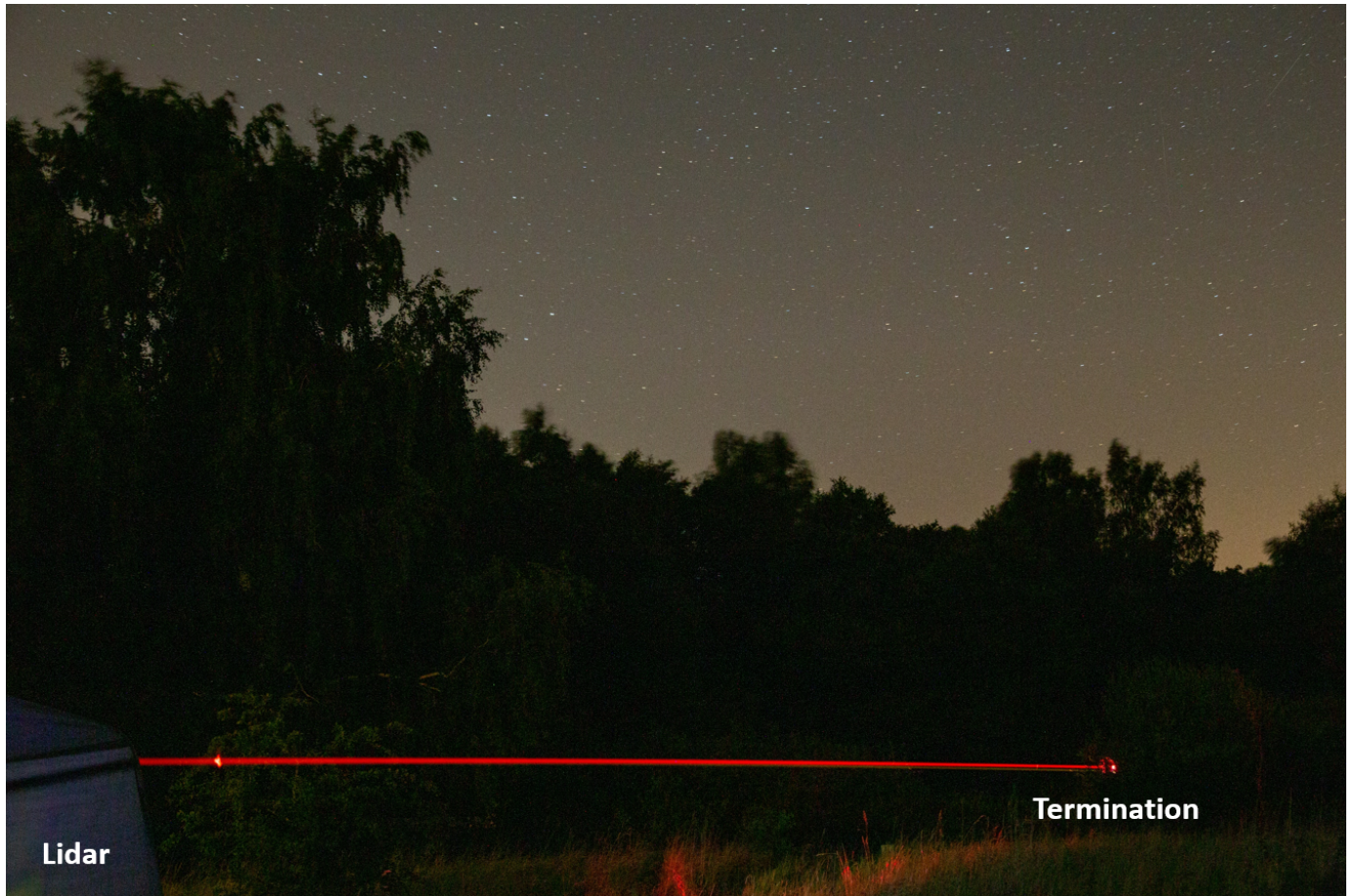
Figure 29: EHS� during field measurement at Stensoffas field station with the super continuum laser beam pointing at the termination.
