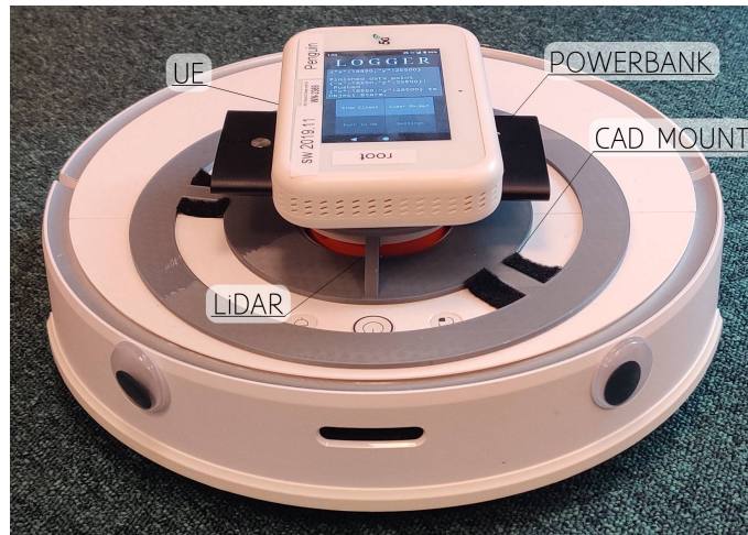
Figure 3.2: Overview of robot used for navigation.
