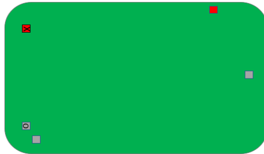
Figure 9.13: Blocked case (Horizontal) – 28 GHz: A mobile device with 1 antenna placed at the back panel and on the right side are active, while the antenna placed at the front panel, 1 on the left-side and 1 at the bottom side are blocked
