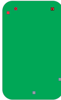
Figure 9.11: Blocked case (Vertical) - 28 GHz: A mobile device with 1 antenna placed at the front panel, 1 at the back panel, 1 on the left-side are active, while the antenna placed on the right-side and 1 at the bottom side are blocked
