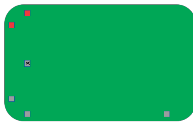
Figure 9.19: Blocked case (Horizontal) - 39 GHz: A mobile device with 1 active antenna on the right side, 1 active antenna on the top side, while the antenna placed at the back side, 2 antennas on the left side and 1 antenna on the top side are blocked
