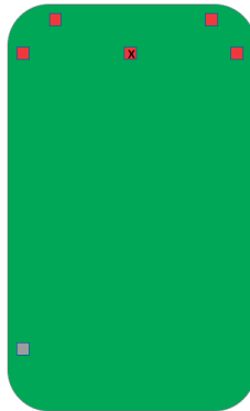
Figure 9.17: Blocked case (Vertical) - 39 GHz: A mobile device with 2 active antennas placed on the top side, 1 active antenna at the back panel, 1 active antenna on the right side, 1 active on the left-side (up) and 1 blocked antenna on the left-side (down)
