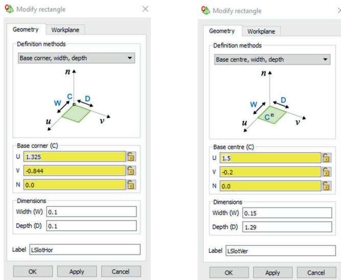
Figure 6.10: Geometry of Horizontal and Vertical slots
