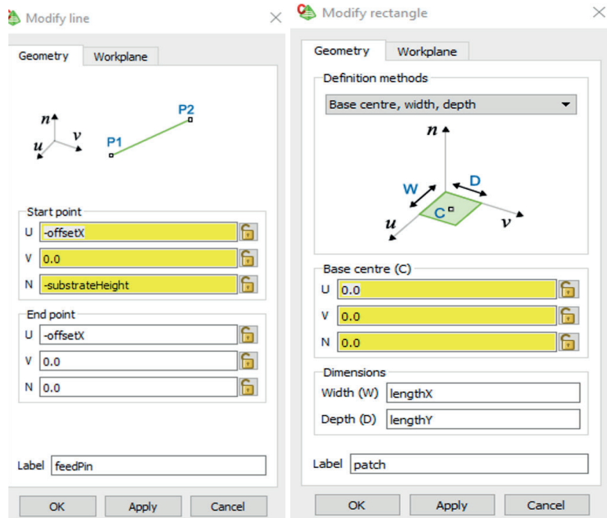
Figure 6.4: Geometry of feed pin and patch antenna
