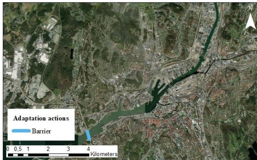
Figure 1. Suggested adaptation action for Gothenburg, riverbank protection by sea walls and a river barrier regulating Göta älv.
