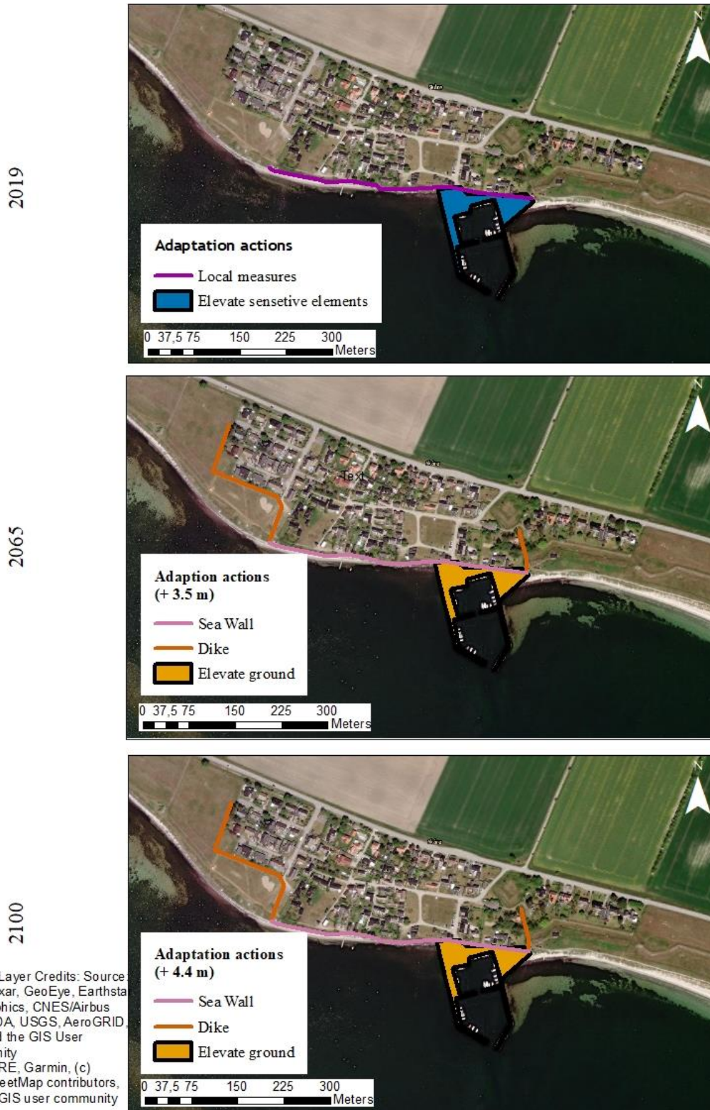
Figure 9. Suggested adaptation actions for Skåre 2019, 2065 and 2100 consisting of local measures, elevation of sensitive elements, dikes, and sea walls.
