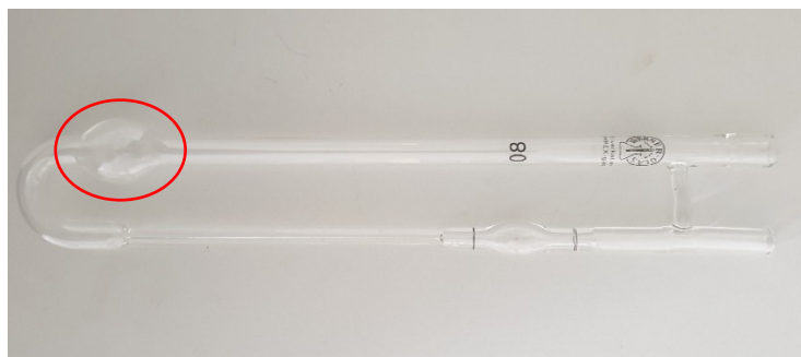
Figure 3.6. The employed Ostwald viscometer, where the two test lines are visible on both sides of the measurement bulb. Encircled is the reservoir bulb of the Ostwald viscometer.
