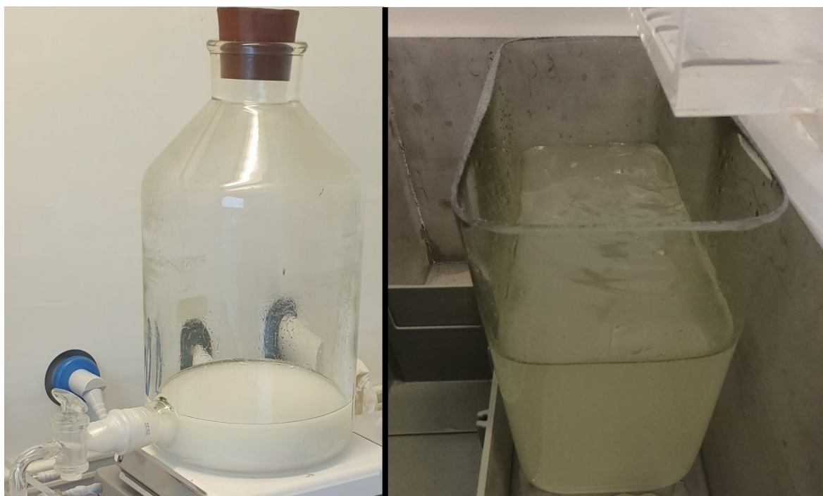
Figure 4.5. Image showing the ingoing (left) and outgoing (right) mixtures to the lamella sedimentation basin.
