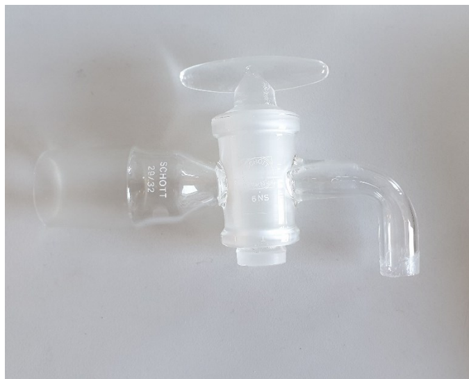
Figure 3.5. The utilized glass stopcock, which enabled the inflow to the lamella sedimentation basin to be regulated.
