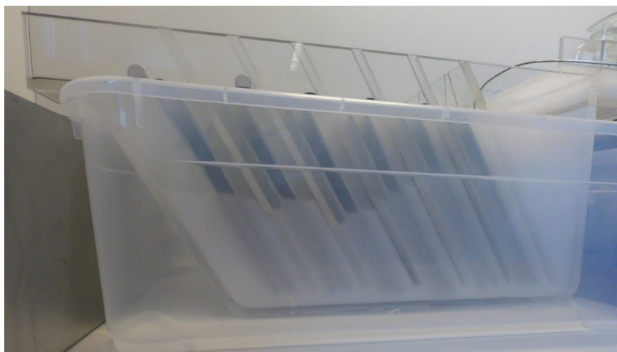
Figure 4.6. The lamella sedimentation basin during operation. The interface between the precipitate-enriched slurry and the lean slurry with less salt crystals can clearly be seen at the distinct border between the white and the more transparent liquid phases.
