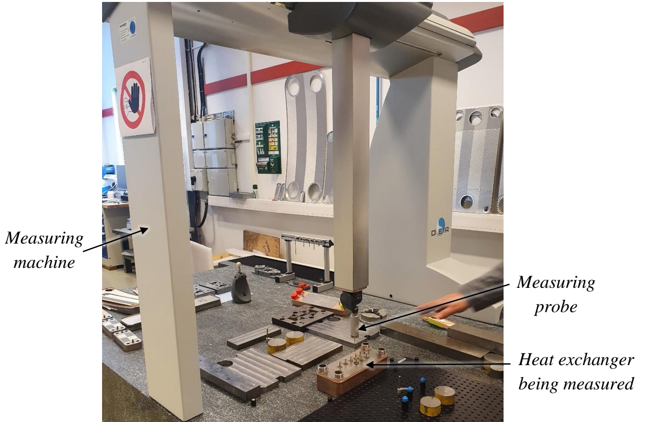
Figure 39: The machine used in the lab to measure the bolt position accuracy
