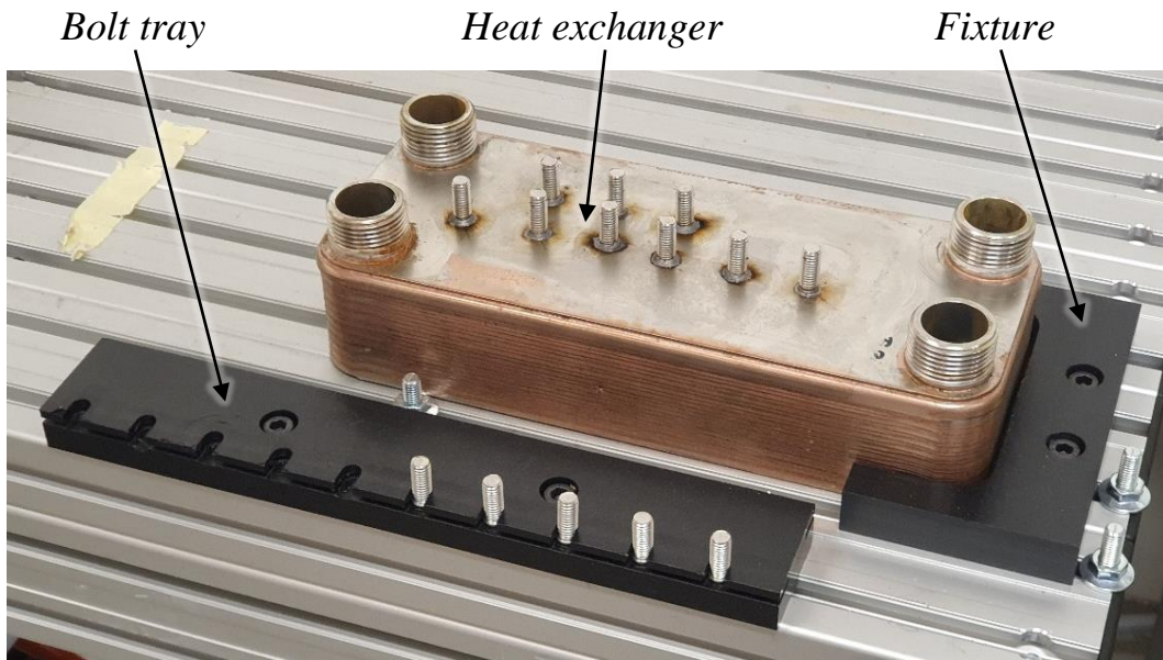
Figure 12: Workstation setup with bolt tray and fixture
