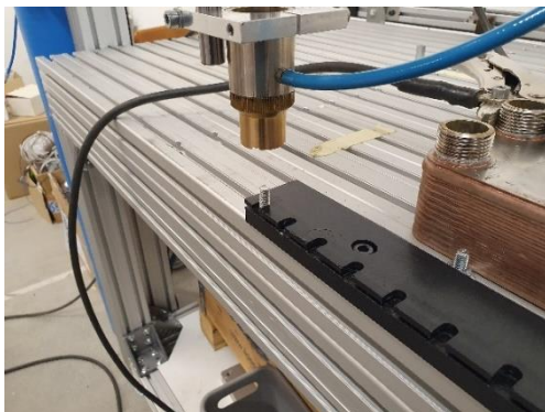
(a) Weld gun above bolt tray position
