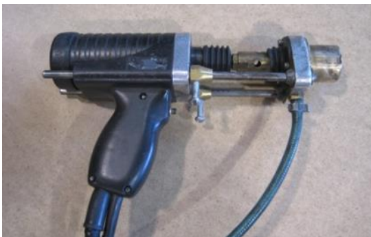
Figure 7: The manual weld gun used
