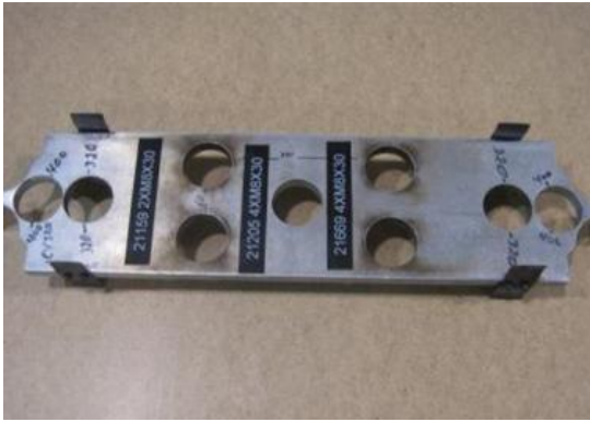
Figure 5: The steel template used to position bolts
