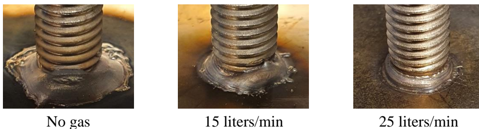
Figure 34: The weld quality tests, varying the gas flow
