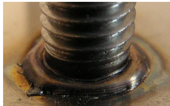
Figure 8: Example of a successful bolt weld
