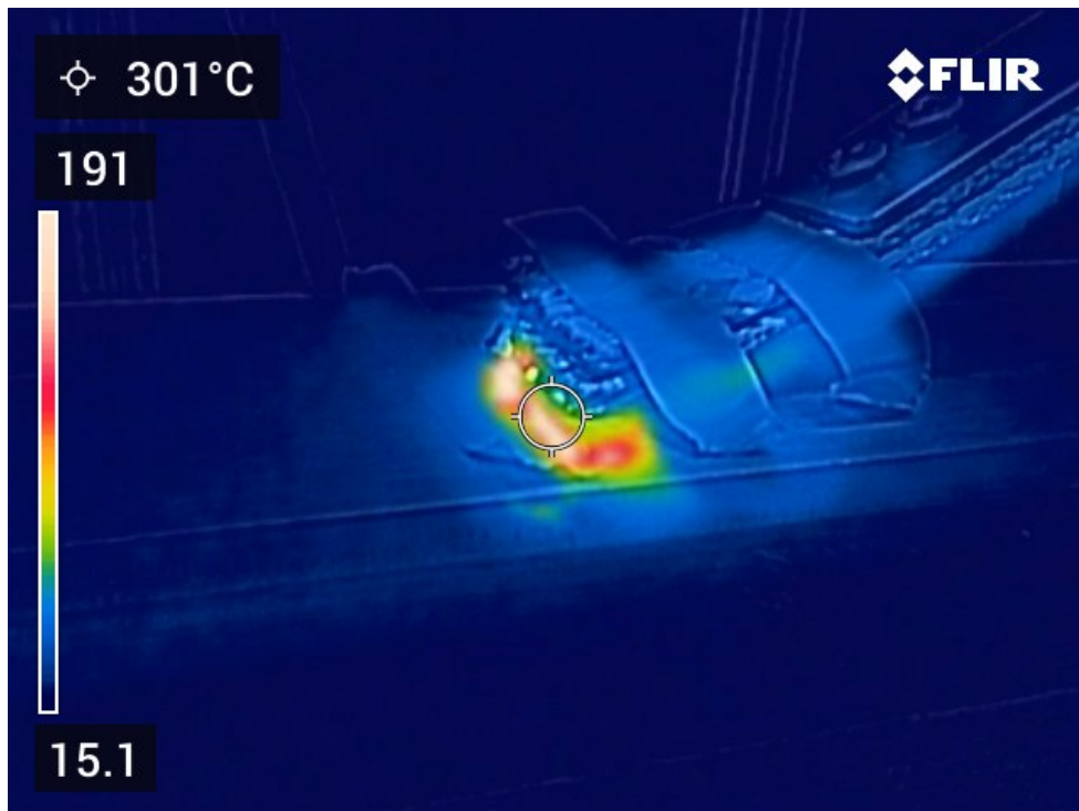
Figure 78. Heat measured during the current conductive test.
