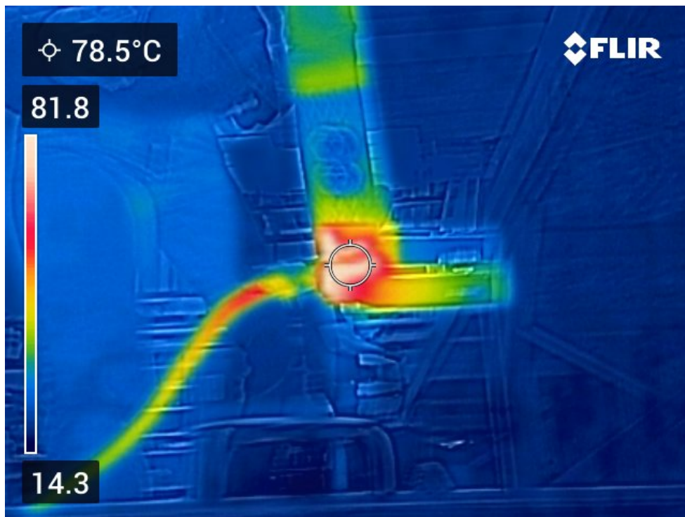
Figure 126. 78.5°C when conducting 143A, stainless steel.
