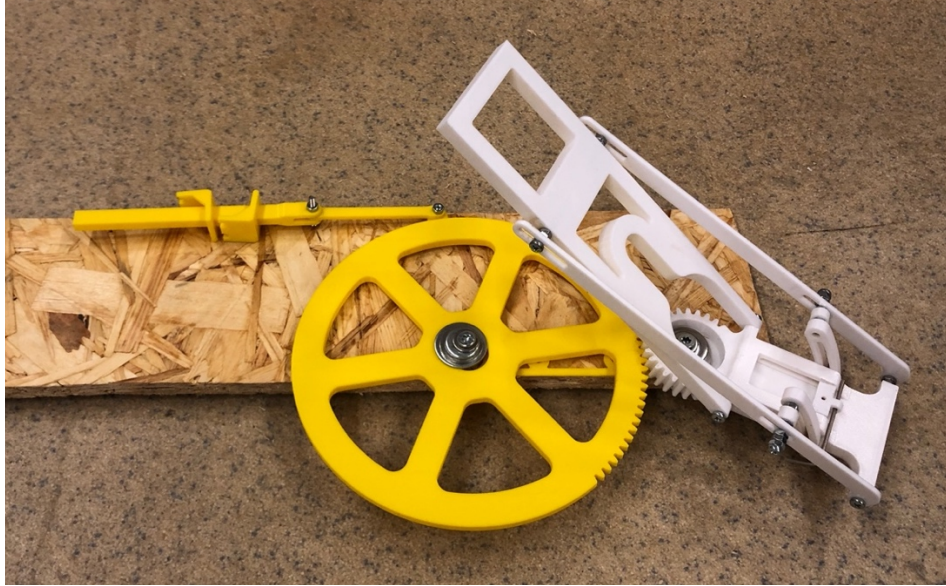
Figure 34. Prototype of the final concept with rotation and folding beam.
