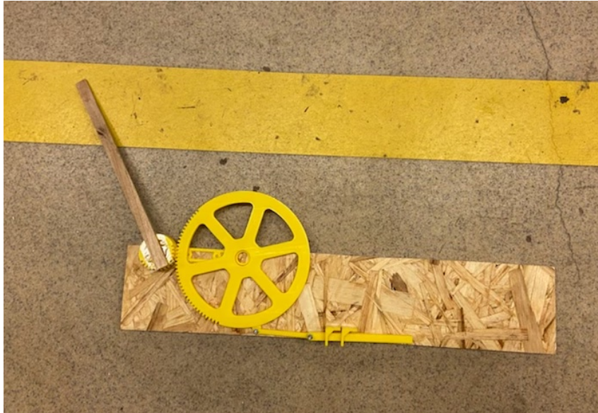
Figure 32. Test of rotational movement using gears.
