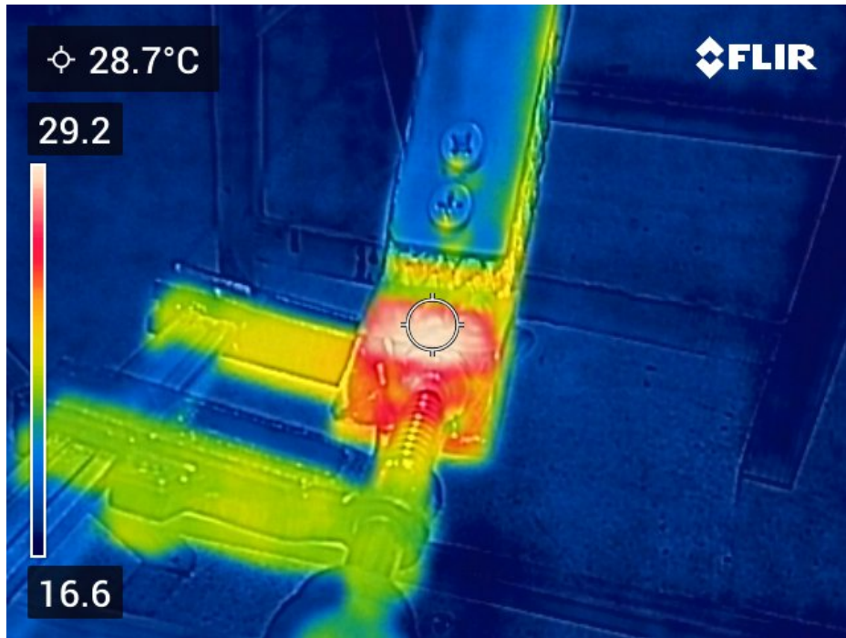
Figure 128. 28.7°C when conducting 143A, copper braid.
