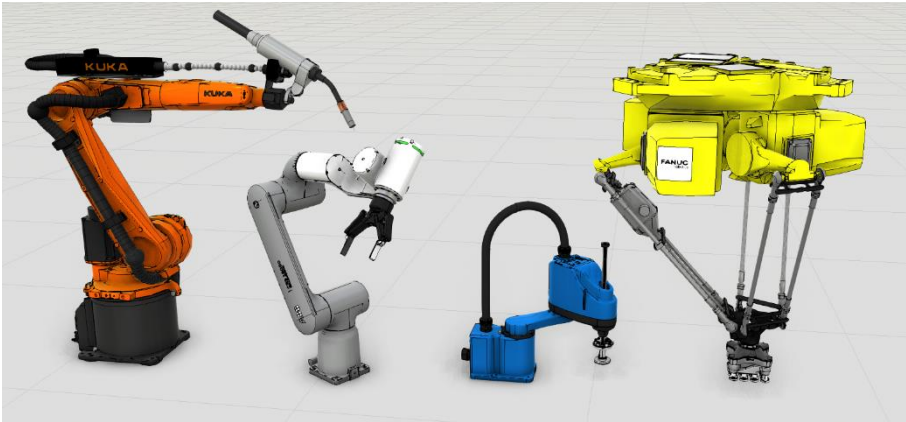
Figure 14 Different robot types from the four largest robot companies. From left, KUKA 6-axis industrial robot, ABB 6-axis collaborative robot, Yaskawa 4-axis SCARA robot, and Fanuc 4-axis Delta robot.
