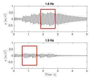
Figure 3. Acceleration response for two different walking frequencies. The 1 s of highest response was determined by calculating the RMS value for all 1 s intervals during the entire five second measurement period and choosing the highest, shown as a red coloured box.
