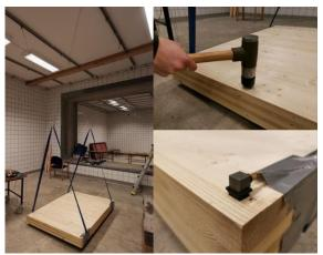
Figure 1. Test setup. The CLT-panel was suspended in the air with rubber bands. An impact hammer was used to induce vibrations in the CLT-panel while the acceleration response was measured.
