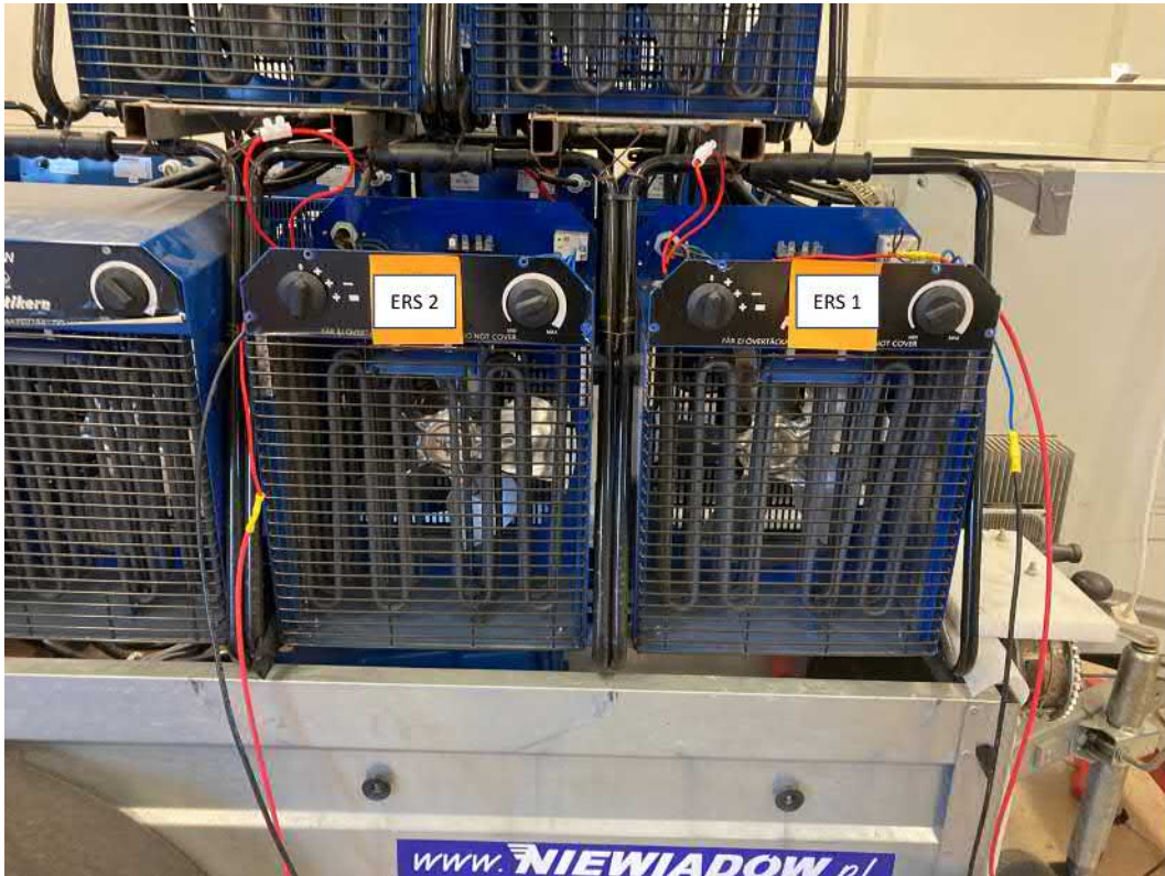
Figure 40: The heating elements used to simulate ERS rails
