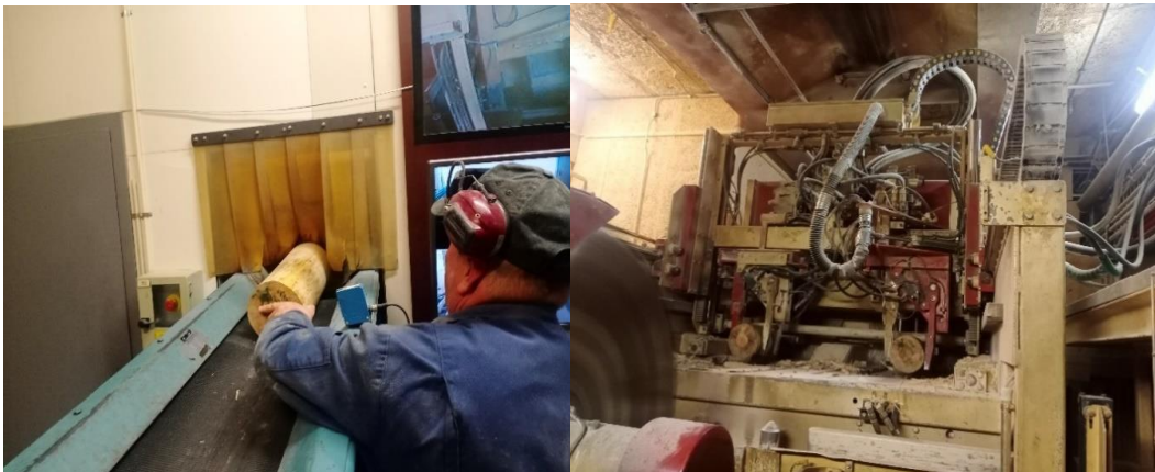
Figure 3.5: Blue pine billet pushing into a shredding machine
