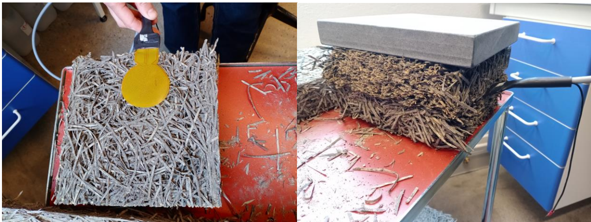
Figure 4.4: Sensor C5599 in between WWS for \lambda -value test
