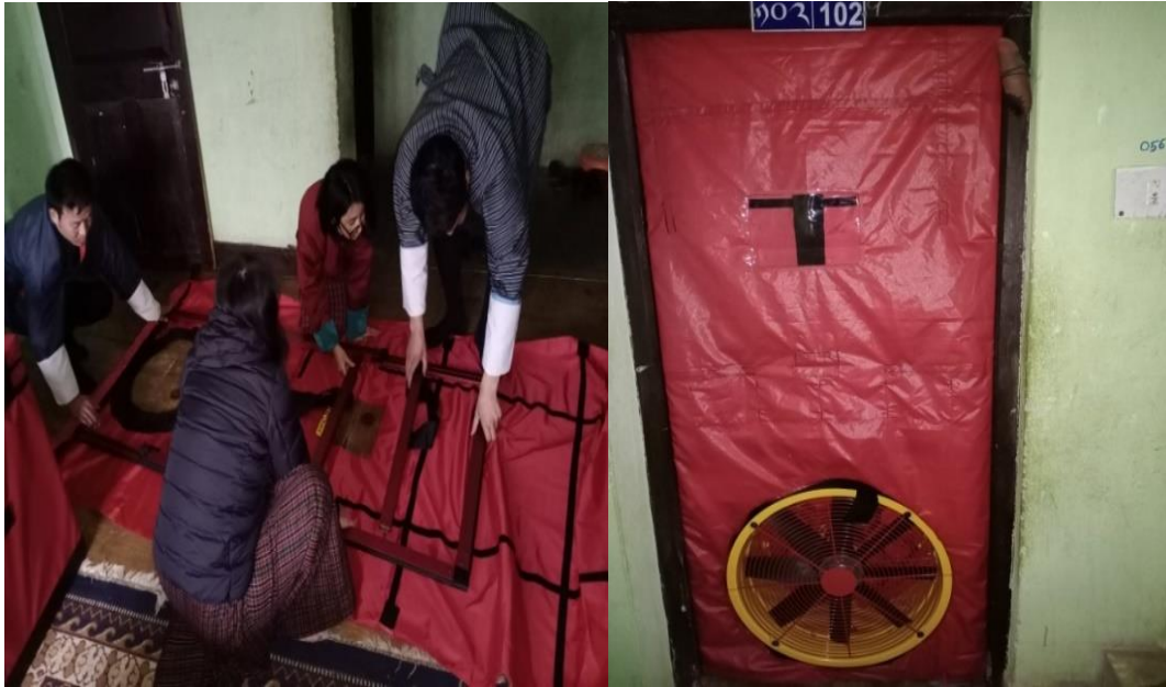
Figure 3.3: Blower door experiment arrangement
