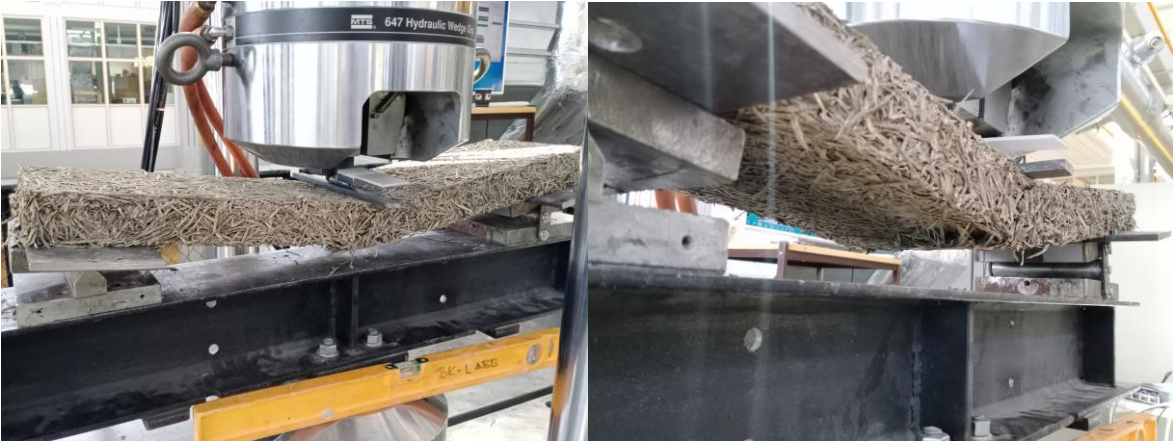
Figure 4.2: Loaded WWS and deformation of the specimen
