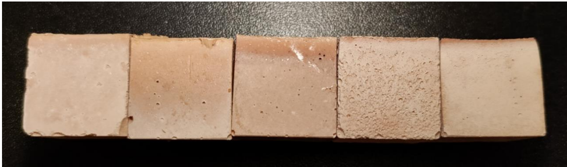
Appendix F Samples of different WTBR from the left 0.31, 0.37, 0.46, 0.57, 0.7
