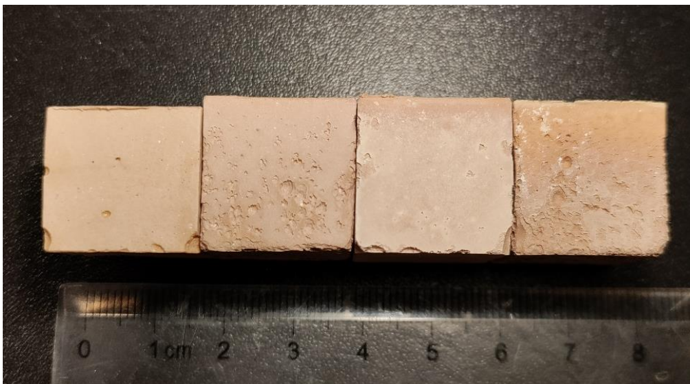
Appendix E Samples cured at different temperatures from the left: 20°C, 40°C, 60°C and 80°C
