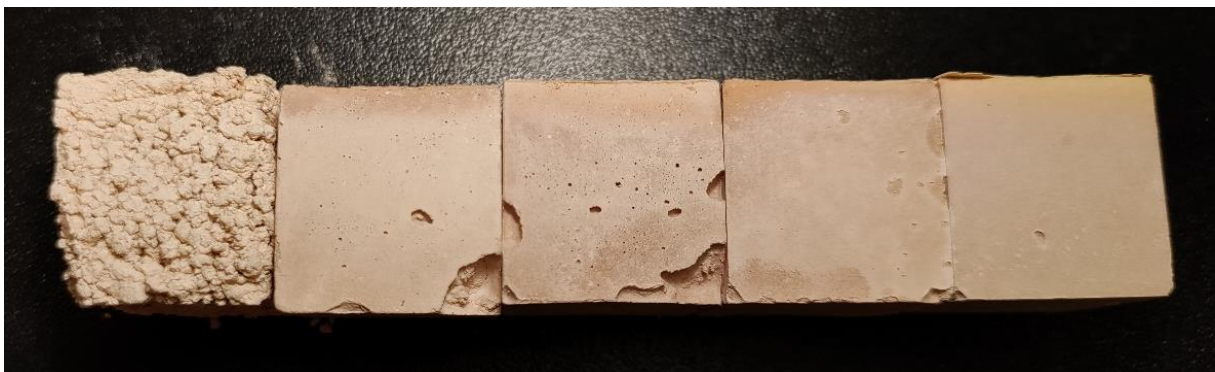
Appendix G Samples with different SoSi content from the left, 4%, 8%, 13%, 21% and 26%
