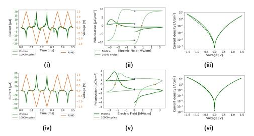
Figure 4.5: The PUND response with calculated PE curve and IV graph for the reference samples with, R (i) - (iii), and without, Ru (iv) - (vi), the oxygen plasma ashing step. The purple and orange dots in the PE curves display the curves' intersect with E=0 and P=0, and can thus be an indication of the remnant polarisation and coercive field.
