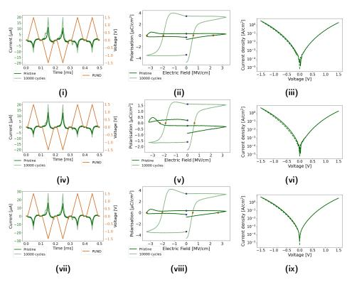
**Figure 4.7:** The PUND response with calculated PE curve and IV graph for sample A1T (i)-(iii), A2T (iv)-(vi), and A3T (vii)-(ix). The purple and orange dots in the PE curves display the curves' intersect with E=0 and P=0, and can thus be an indication of the remnant polarisation and coercive field.
