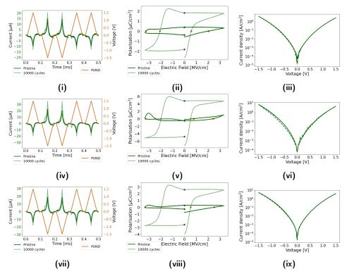
**Figure 4.8:** The PUND response with calculated PE curve and IV graph for sample B1T (i)-(iii), B2T (iv)-(vi), and B3T (vii)-(ix). The purple and orange dots in the PE curves display the curves' intersect with E=0 and P=0, and can thus be an indication of the remnant polarisation and coercive field.
