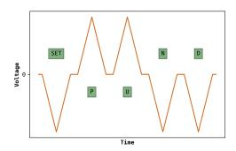
$\textbf{Figure 2.13:} \ \, \textbf{The voltage scheme used in PUND measurements}.$
