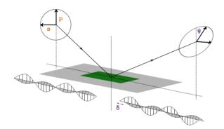
**Figure 2.12:** The change in polarisation upon reflection on a sample. This is utilised in spectral ellipsometry.
