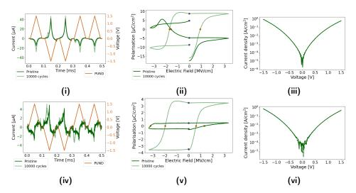
**Figure 4.10:** The PUND response with calculated PE curve and IV graph for sample C1T (i)-(iii) and C2T (iv)-(vi). The purple and orange dots in the PE curves display the curves' intersect with E=0 and P=0, and can thus be an indication of the remnant polarisation and coercive field.
