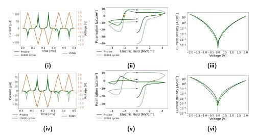
**Figure 4.11:** The PUND response with calculated PE curve and IV graph for sample D1B (i)-(iii) and D2B (iv)-(vi). The purple and orange dots in the PE curves display the curves' intersect with E=0 and P=0, and can thus be an indication of the remnant polarisation and coercive field.
