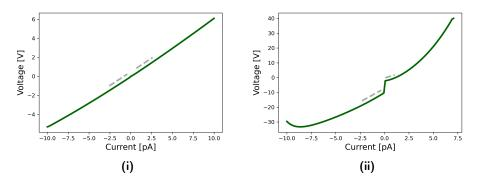
**Figure 4.4:** The sourced current and measured voltage from four-probe measurement of two of the samples; **i** exhibiting an ohmic and **ii** non-ohmic relation. The gray dashed lines indicates the datapoints used to measure the resistance.
