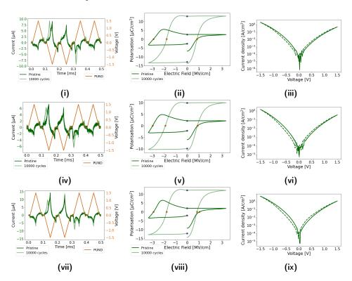
**Figure 4.6:** The PUND response with calculated PE curve and IV graph for sample A1B (i)-(iii), A2B (iv)-(vi), and A3B (vii)-(ix). The purple and orange dots in the PE curves display the curves' intersect with E=0 and P=0, and can thus be an indication of the remnant polarisation and coercive field.
