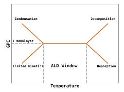
**Figure 2.9:** A schematic of the dependence of the growth per cycle (GPC) on the deposition temperature. The figure shows a temperature interval of constant GPC of 1 monolayer, called the ALD window.
