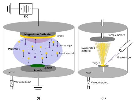
Figure 2.11: A schematic of (i) a sputterer and (ii) an electron beam evaporator used for thin film deposition.
