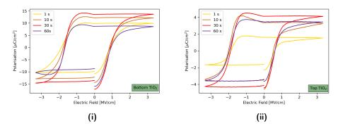
**Figure 4.15:** The PE curves from the **(i)** bottom  $TiO_2$  and **(ii)** top  $TiO_2$  samples of varying plasma exposure time in the  $TiO_2$  ALD deposition. The other deposition parameters were identical. The data from samples A2(B/T), A3(B/T), C1(B/T), and C2(B/T) was used.
