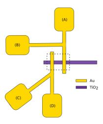
Figure 3.2: The gold structure used for four-probe measurements on the  $TiO_2$  strip
