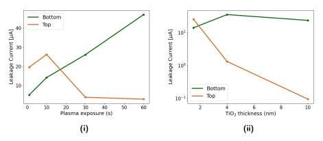
Figure 4.14: The leakage current as function of the (i) plasma exposure and (ii)  $TiO_2$  thickness. The current was measured during the negative IV sweep at -1.5 V.
