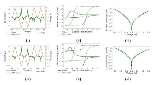
**Figure 4.9:** The PUND response with calculated PE curve and IV graph for sample C1B (i)-(iii) and C2B (iv)-(vi). The purple and orange dots in the PE curves display the curves' intersect with E=0 and P=0, and can thus be an indication of the remnant polarisation and coercive field.
