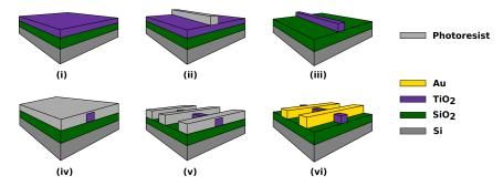
**Figure 3.1:** Illustration of the sample structures during different stages in the processing. The TiO<sub>2</sub> layer thickness was around 10-20 nm; The dimensions are not to scale.
