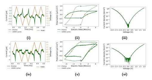
**Figure 4.12:** The PUND response with calculated PE curve and IV graph for sample D1T (i)-(iii) and D2T (iv)-(vi). The purple and orange dots in the PE curves display the curves' intersect with E=0 and P=0, and can thus be an indication of the remnant polarisation and coercive field.
