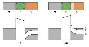
**Figure 2.5:** Schematic of the metal-ferroelectric insulator-semiconductor (MFS) heterostructure and the corresponding bandstructure at the two polarisation states of the ferroelectric. The semiconductor is n-doped.
