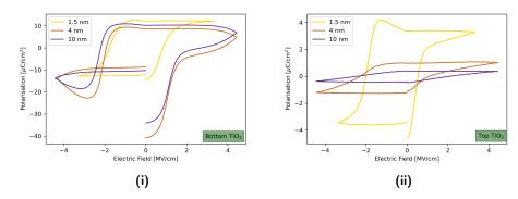
**Figure 4.16:** The PE curves from the **(i)** bottom  $TiO_2$  and **(ii)** top  $TiO_2$  samples of varying  $TiO_2$  thickness in the  $TiO_2$  ALD deposition. The other deposition parameters were identical. The data from samples A3(B/T), D1(B/T), and D2(B/T) was used.
