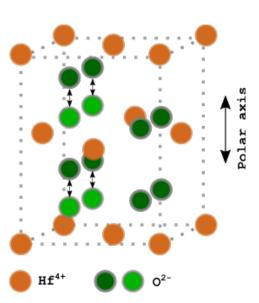
**Figure 2.4:** The ferroelectric orthorombic phase of HfO<sub>2</sub>. The figure shows two equilibrium positions of the oxygen ions in the lattice resulting in two polarisation states along the polar axis.
