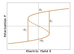
Figure 2.3: Polarisation as a function of electrical field including the remnent polarisation  $\mathsf{P}_R$  and coercive field  $\mathsf{E}_C$ .
