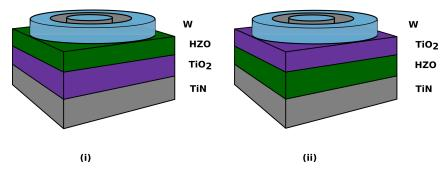
**Figure 3.3:** The heterostructure of the FTJs constructed in this thesis. The difference between the two images is the placement of the TiO<sub>2</sub> layer. Dimensions are not to scale.
