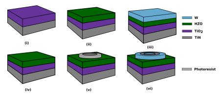
**Figure 3.4:** Illustration of the FTJ sample structure during different stages in the processing. Important to note is that the  $TiO_2$  is placed beneath the HZO layer, *i.e.* a bottom  $TiO_2$  FTJ.
