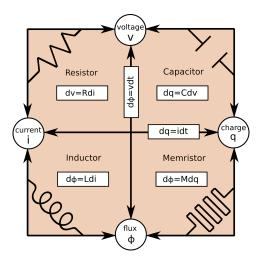
**Figure 2.7:** The four fundamental two-terminal circuit elements; the resistor, capictor, inductor, and the memristor. The figure show their relationship to each other via the state variables.
