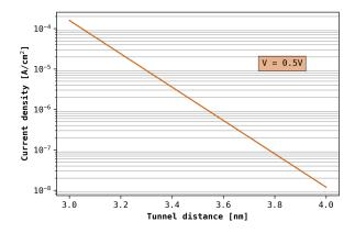
Figure 2.6: The current density as a function of the tunnel distance at an applied voltage of 0.5V. The following parameters are used in the simulation:  $\Phi_{B,1}=\Phi_{B,2}=1e\text{V}$ , and  $m_{e,oxide}=m_e=9.109E-31\text{kg}$
