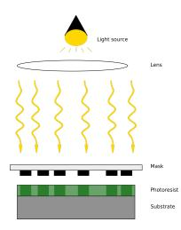
**Figure 2.10:** Illustration of the patterning of a light sensitive material in photolithography.
