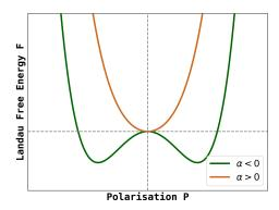
**Figure 2.1:** The Landau free energy as a function of polarisation given by equation 2.3 and E=0.
