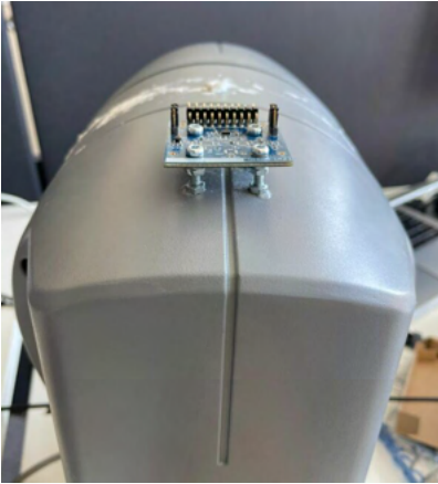
Figure 6.5 IMU mounted on moving part of camera for vibration tolerance test.
