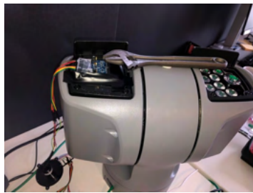
Figure 3.5 Setup when testing magnetometer with disturbance present.
