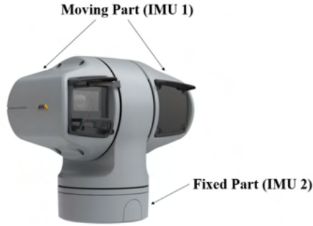
Figure 6.2 Axis Q6215 camera showing the possible placements of the moving and fixed IMU.
