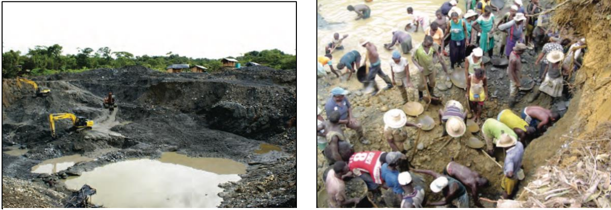
Figure 15: mechanized mining (left) and artisanal mining (right) are carried out in the same river (Sarmiento et al., 2013)
