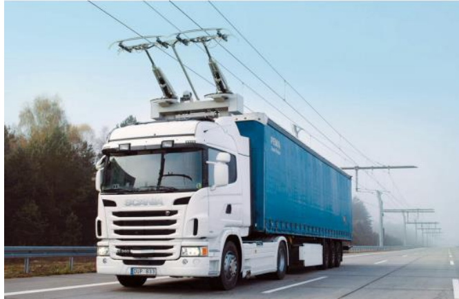
Figure 2. Truck driving with Siemens' overhead lines technology (Energipress 2015)
