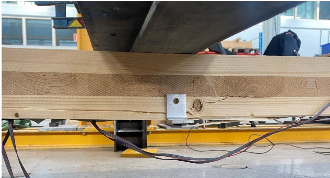
Figure 4.12: Cracks in the slab at maximum load
