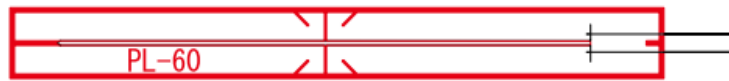
Figure 2.11: Figure of the strain gauge used in the tests, the figure was used with permission from Tokyo Measuring Instruments Lab (n.d.-b)
