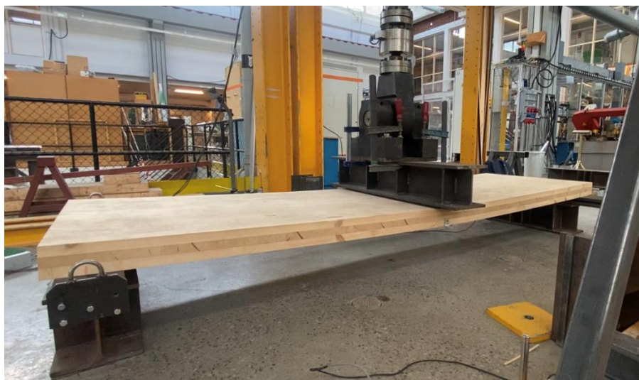
Figure 4.13: The deflection of the slab at maximum load.
