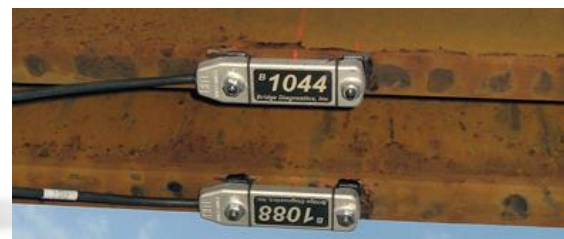
Figure 2.13: A depiction of the ST350 Strain transducer from BDI (n.d.) in use.
