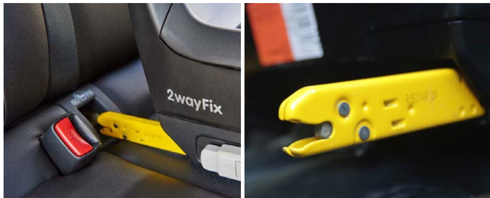
Figure 3: Left: ISOfix car seat installation (Monson 2022). Right: ISOfix mount (NFT 2022)
