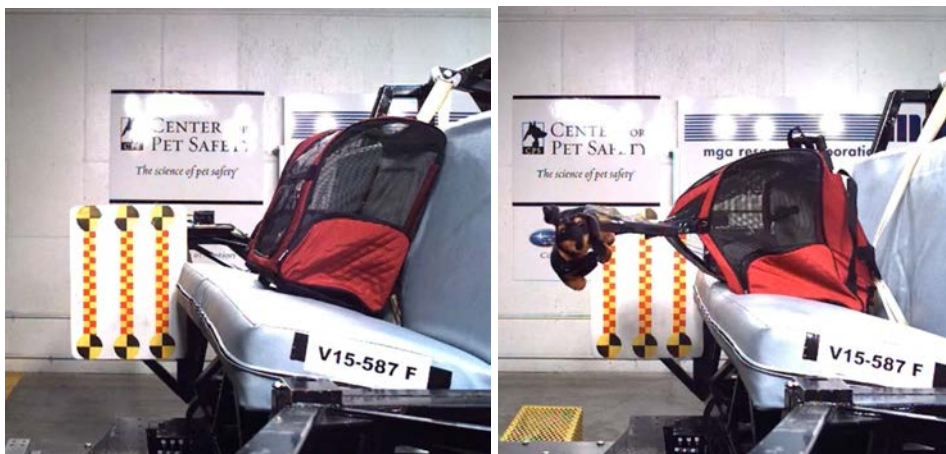
Figure 15: How the placement of a zipper affects a crash (Centre for Pet Safety, 2020)
