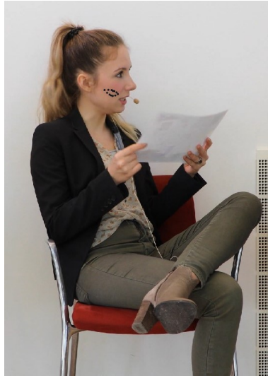
Figure 5.1 A frame of an actor with black dots on the frame representing the coordinates of the landmarks created by the algorithm of where it thinks the mouth is supposed to be.
