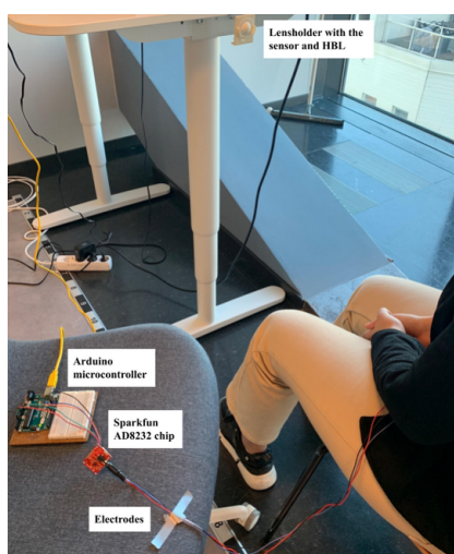
(a) An overview of the measurement setup, where the use of the radar sensor and the ECG can be seen.
