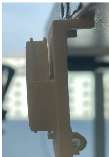
(b) The lens holder horizontally attached to the table.
