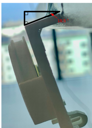
(a) The lens holder is tilted with an angle of 18 degrees.
