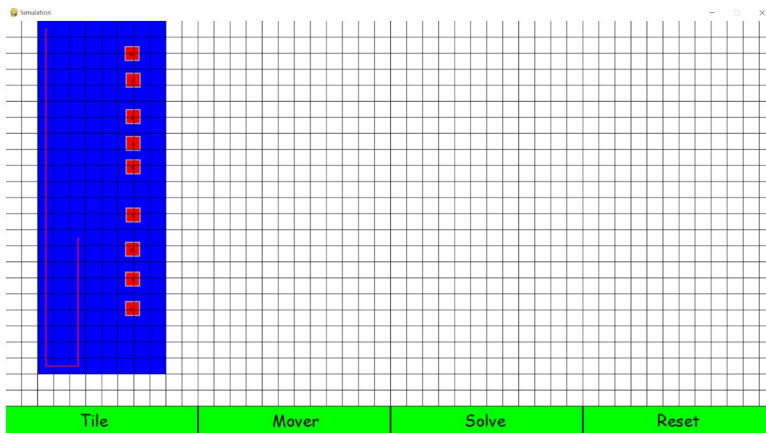
Figure 3.1 illustrates the GUI for the simulation package. Blue colouring indicates the tiles, red squares indicate the movers, grid elements represent nodes in the configuration space and the red line indicates the specified startup-path for movers to align on.
