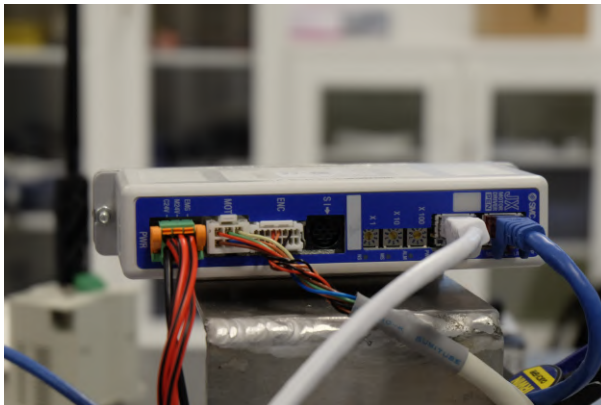
Figure 2.8 Servo driver connected over Ethernet/IP
