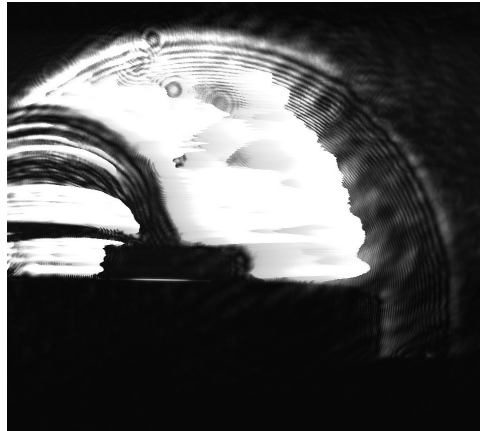
Figure 26: The output facet of an Optical Tapered Amplifier (OTPA), imaged with a microscope objective (PLN 4X, Olympus) via a Beam-Profiler software developed by Anders Persson, research engineer at the Division of Atomic Physics at Lund University.
