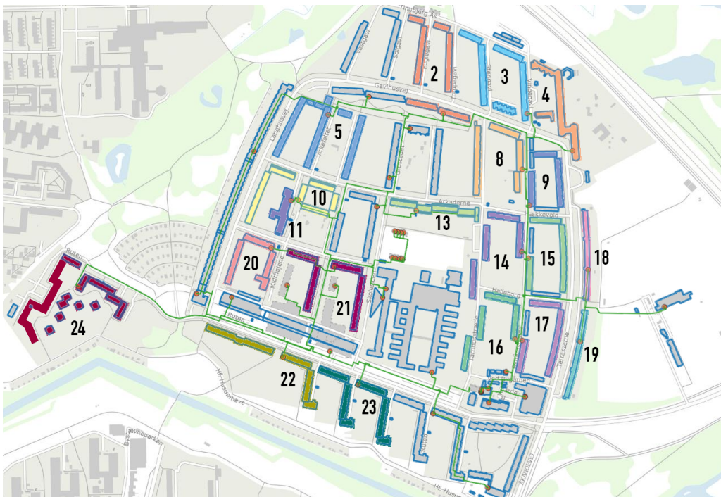
Figure 15: Map of Tingbjerg neighborhood in Copenhagen oriented North. Green lines denote district heating pipes supplying hot water to local heat exchangers (orange dots). Numbers on the image correspond to building groups of the heating exchanger datasets we were able to successfully clean.
