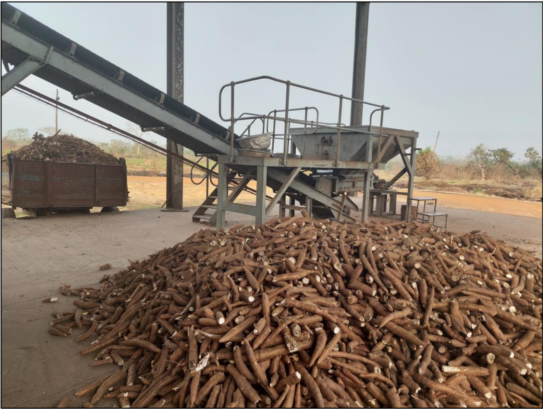
Figure 4. Cassava processing conveyor. Ethanol production company, community 1.
