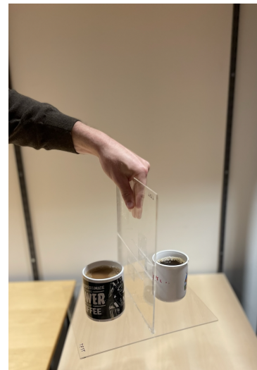
Figure 10. Ad hoc stress test of solvent weld
