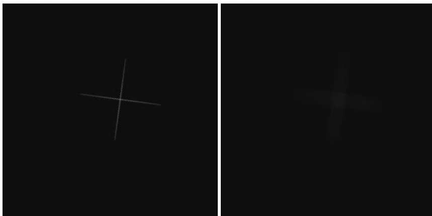
Figure 1.2: The image taken by the sensor during active alignment. The left picture shows when the target is in focus and the right shows when it is not.
