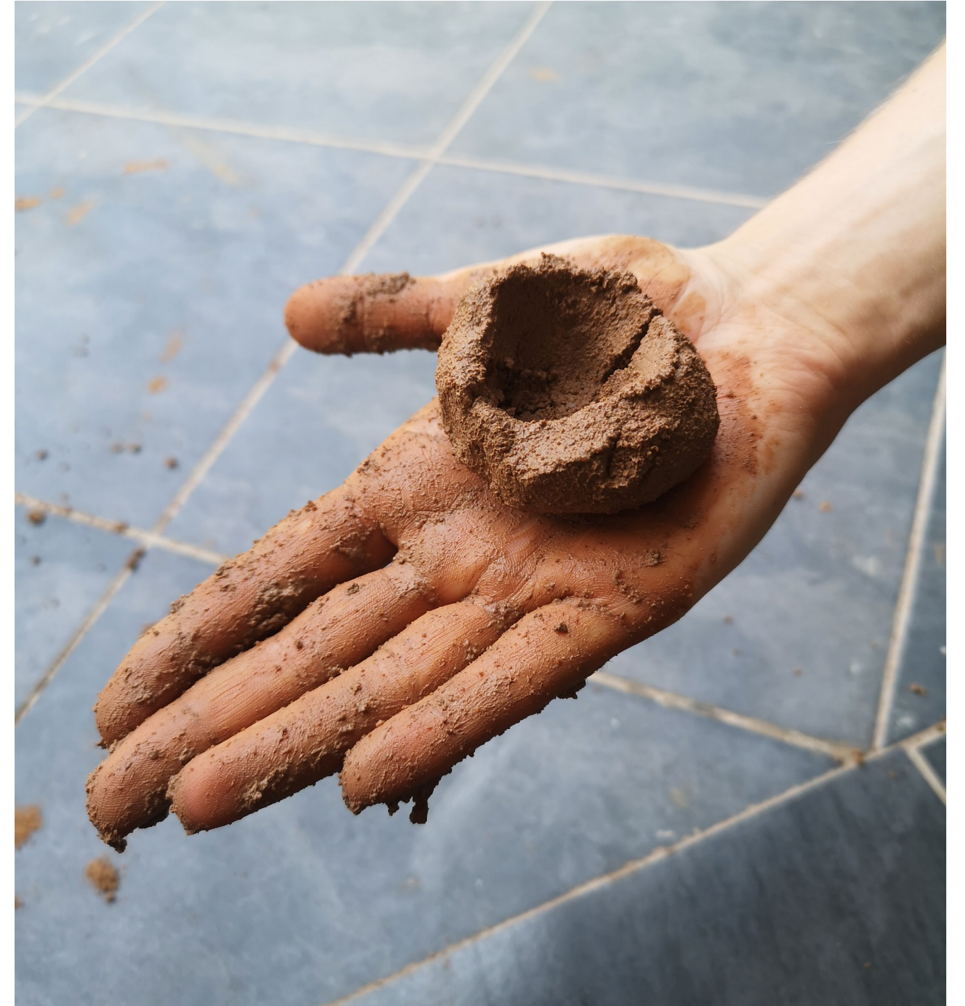
Picture of one of the tests that we conducted. This one shows the beginning of the absorption test, before water is added.
