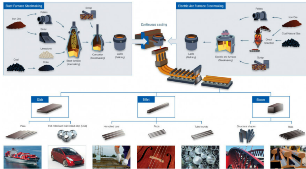
Figure 3.2: BOF and EAF production routes (ESTEP, 2021).
