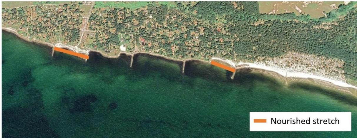
Figure 3.9. The parts of Löderups Strandbad that were nourished during 2020 (Skoog, 2020). Satellite image from GoogleEarth, 2019.
