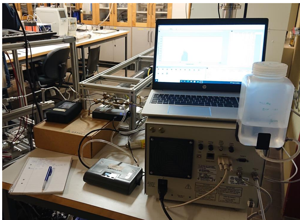
Figure 3.3 Partector 2, Partector TEM, microAeth MA300, and SMPS connected to the thermodenuder.
