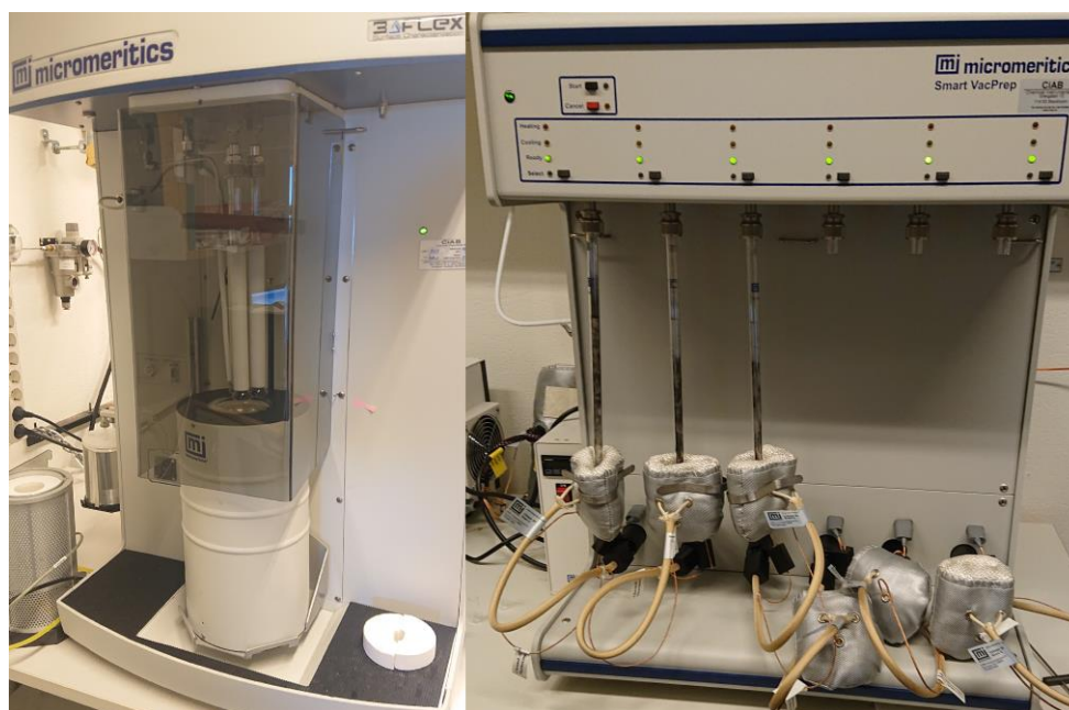
Figure 3.5 On the left: Micromeritics 3Flex surface characterization analyser used for BET reference measurement. On the right: Micromeritics Smart VacPrep used to pretreat samples for the 3Flex.
