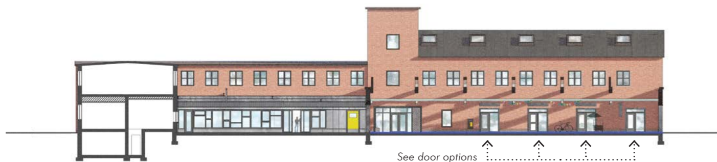
Elevation through passage / 1:400/ North facing courtyard facade - orangery connected to workshop space and commercial passage.
