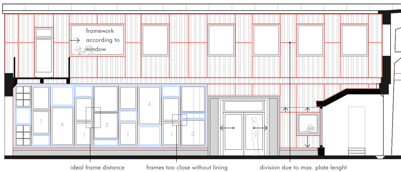
A. Framework system of corrugated plates
