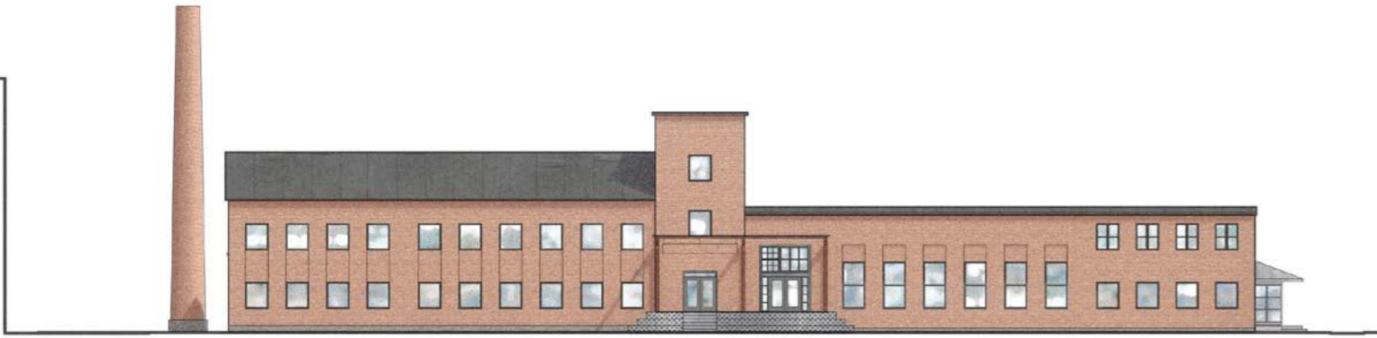
Elevation facing South / 1:400 / Entrance seating stairs in perforated metal, reused window section opening up into the workshop hall.
