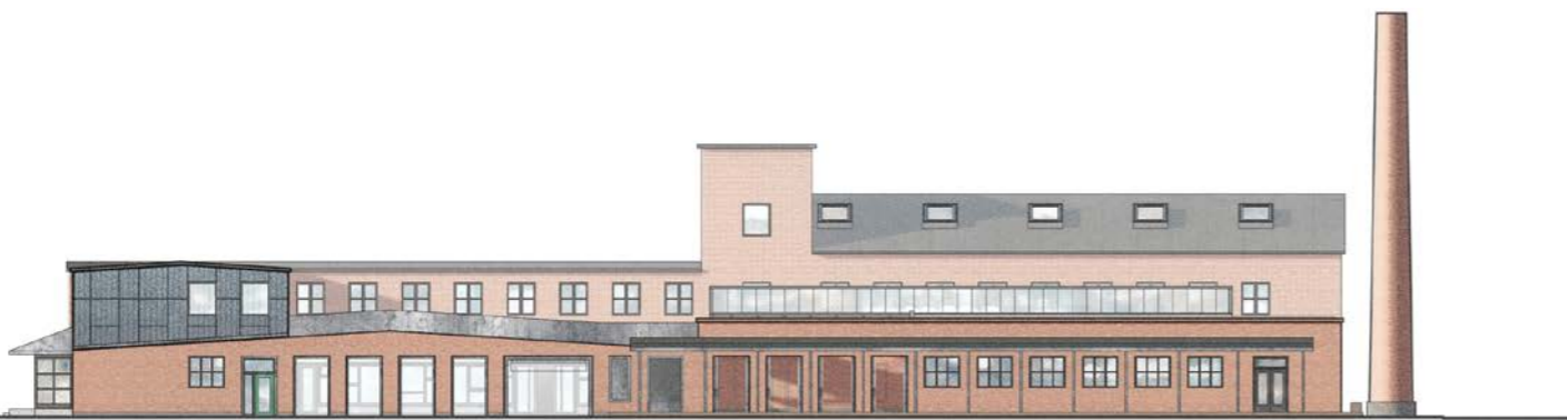
Elevation facing North / 1:400 / Side towards the park - roofed terrace by the café/event hall, viewing platform above the courtyard.
