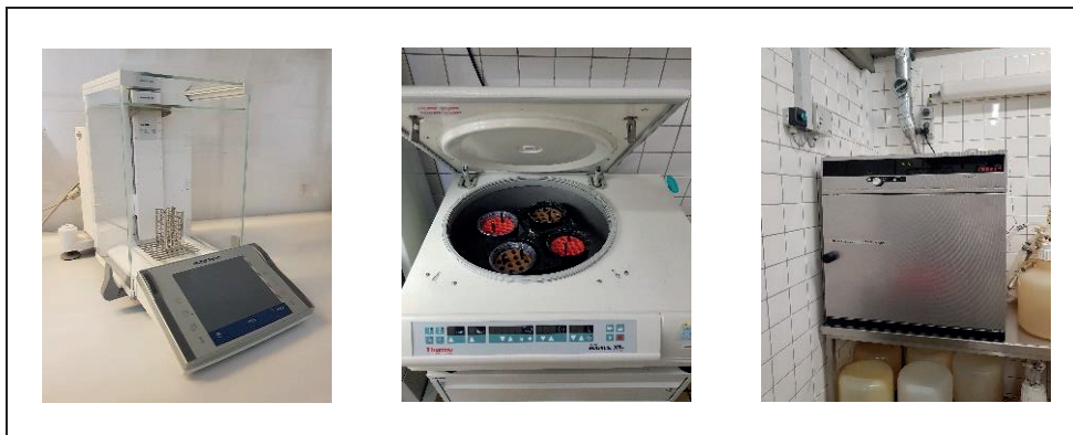
Figure 3.4. Left: XP204 Scale from Mettler Toledo. Middle: Heareus Multifuge 3SR+ centrifuge from Thermo Scientific. Right: Memmert oven from Buch & Holm.
