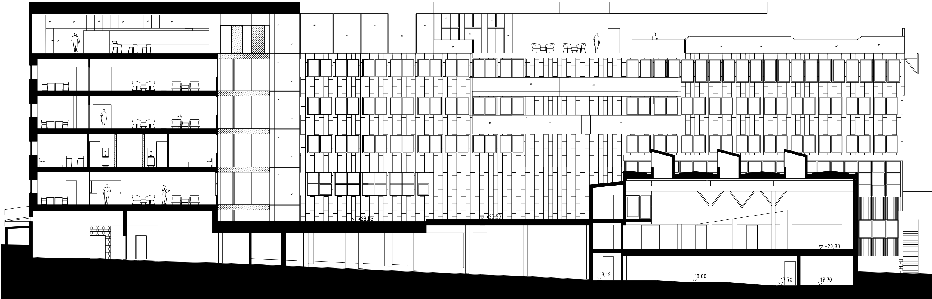
SECTION A-A Connection between the existing building and the additional floor. Section below shows the relation to the opposite building.
