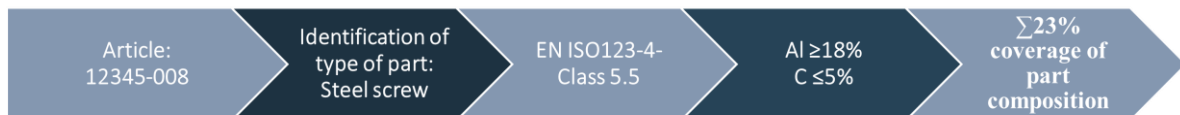
Figure 7. Figure describing the identification and summary process when determining the total chemical composition within components used in the T-15 GPHE business unit using material standards.
