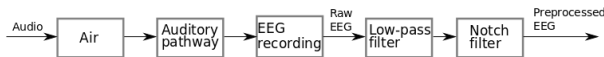
Figure 4.1 A block diagram that shows what has been done with the EEG signals and what they have been affected by.
