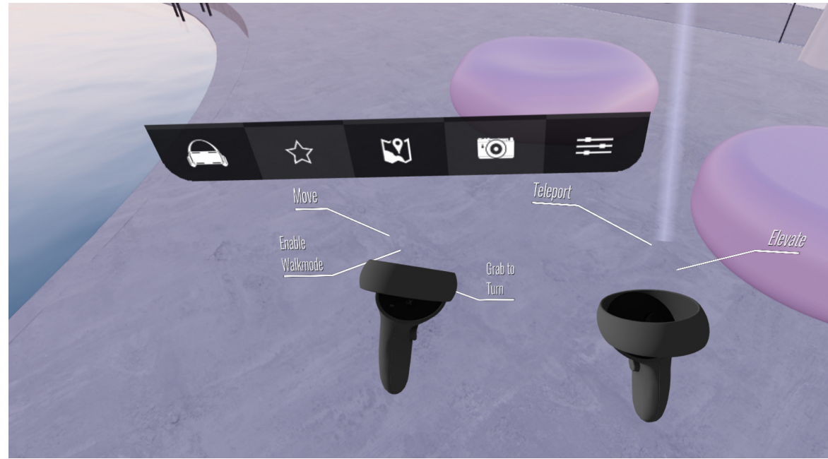
CONTROLLERS The user will be able to view the controllers and a menu when navigating around. The hands/controllers will be shown in VR. The rest of the body is not visible in VR.
