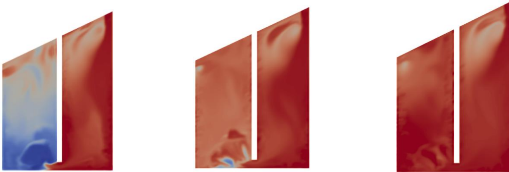
Fig.3.3d: Time, t = 20 mins Fig. 3.3e: Time, t = 30 mins Fig.3.3f: Time, t = 55 mins Figure 3.3: Time taken to reach maximum average temperature in exothermic wall condition.
