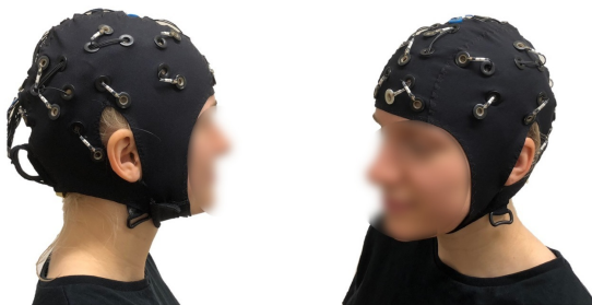
Figure 1.2 An EasyCap 2 EEG cap of size 58 from two different perspectives. The cap has a 24-channel montage, with the purpose of simplifying electrode placement in a consequent manner between subjects.
