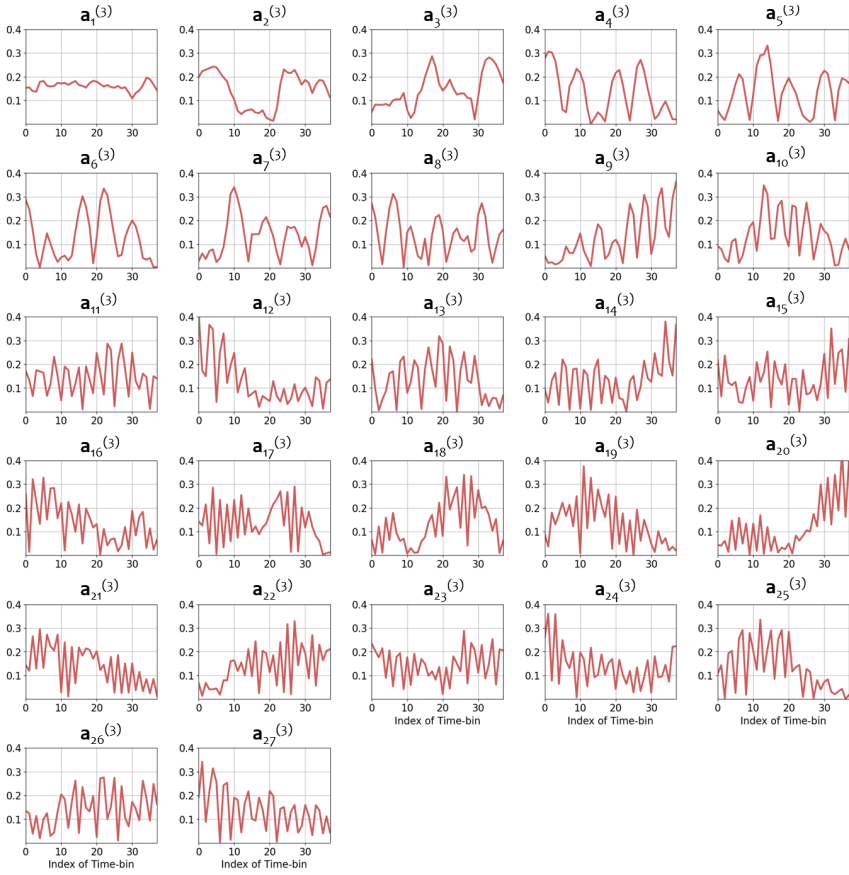
Figure 6.7 Plot of each column of the 6th session's feature space time-factor \mathbf{A}^{(3)} \in \mathbf{R}^{38 \times 27} . The 6th session was thus excluded when computing these factor matrices. Note that the plots present the absolute values of a column. A large value thus corresponds to a large amplitude.
