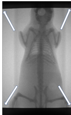
Figure 3.4: Barrel distortion in a cone-beam X-ray projection of the 3D printed mouse phantom. The Barrel distortion is noticeable at the periphery of the cone-beam X-ray projection as indicated by the white arrows.
